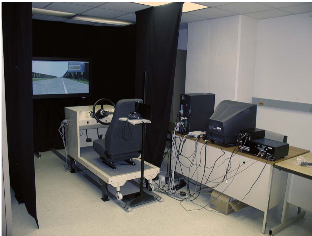
Figure 7. VT-UVA-Carilion driving simulator and experimental environment.
