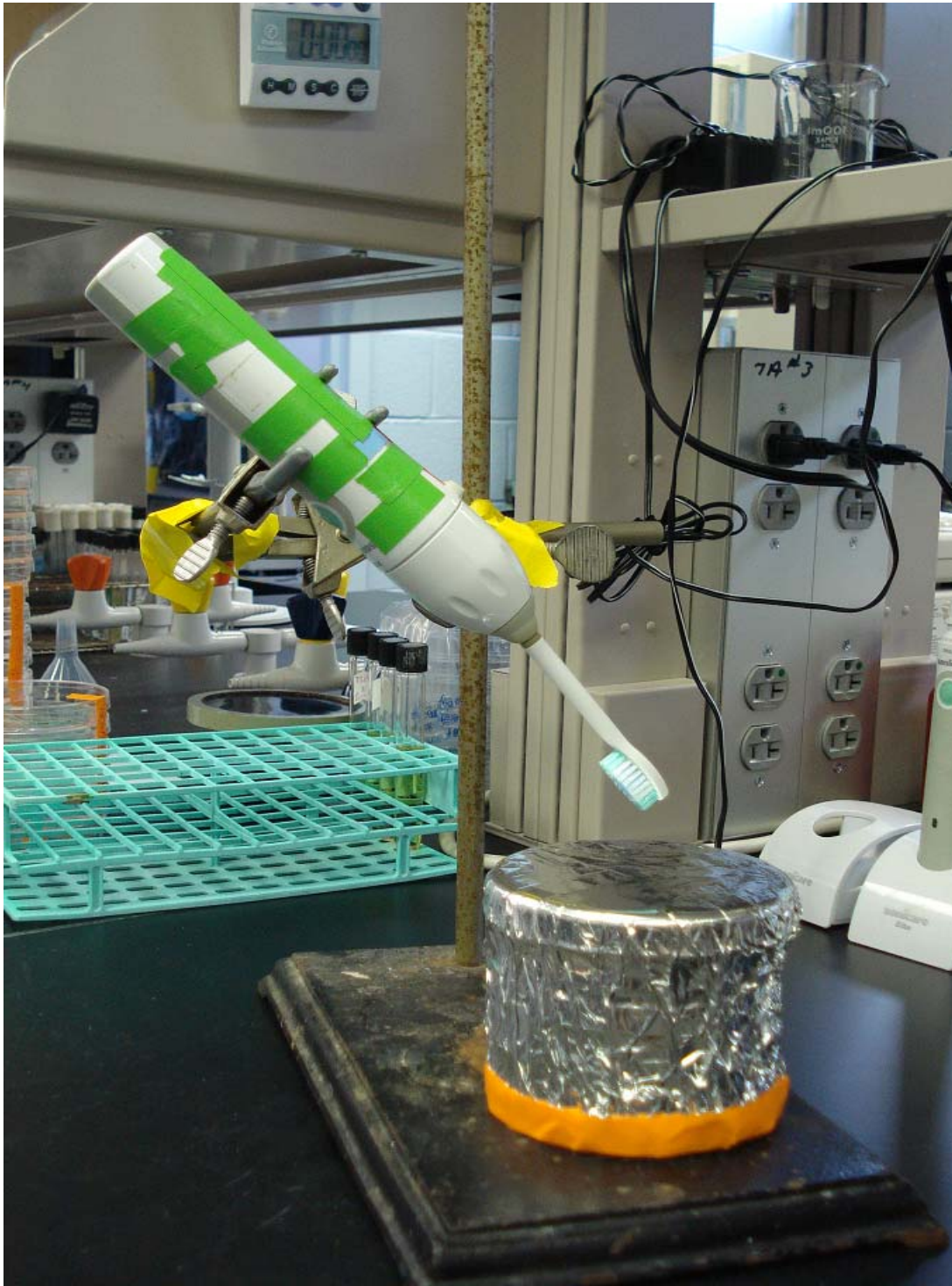
Appendix A, Figure 2. Sonicare® Elite 7300 apparatus for the sonicating brush method.
