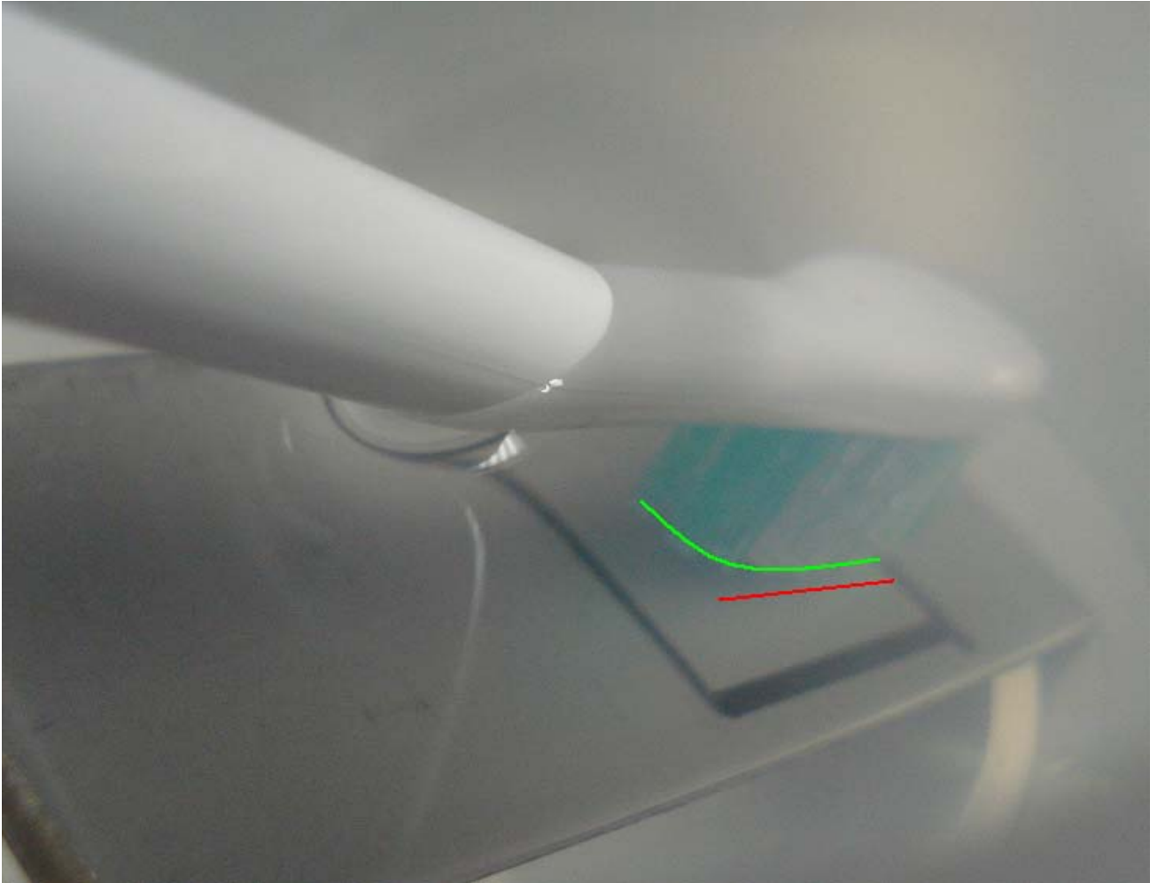
Appendix A, Figure 3. Position of the brush head relative to the inoculated area on the stainless steel coupon submerged in 100 mL PBS solution used for the sonicating brush method.
