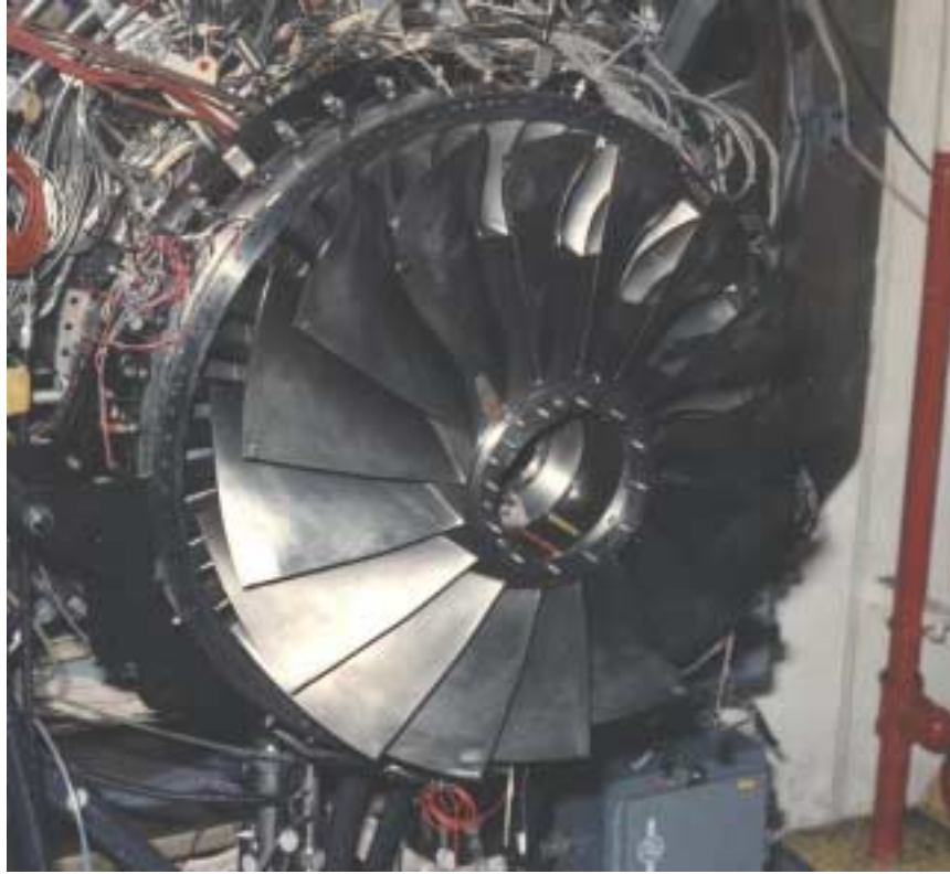
Figure 4.3: First Stage Blisk Mounted in Test Rig
