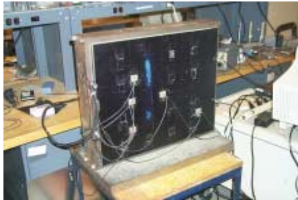
Figure 5.3. The simply supported test plate under investigation.
