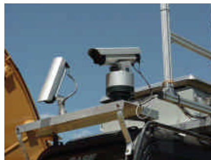
Figure 4-5: Teleoperated front viewing vision system
