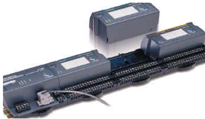
Figure 5-8: FieldPoint modular distributed I/O system [15]
