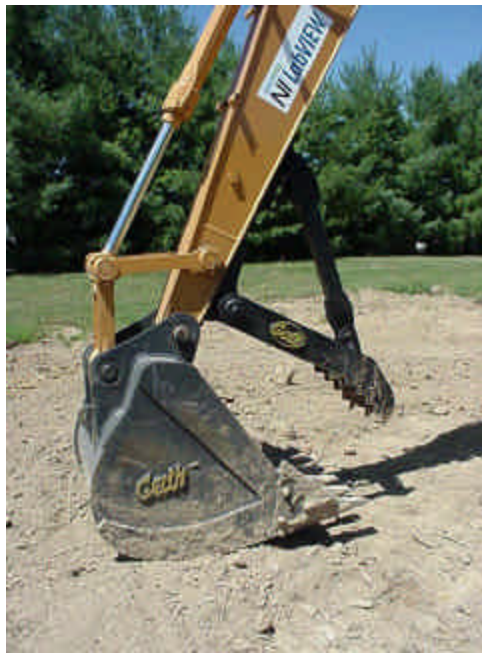
Figure 3-2: Excavator bucket with attached thumb
