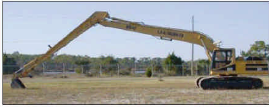
Figure 2-2: Advanced Automated Ordnance Excavator (AAOE) [6]
