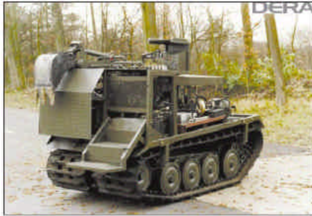
Figure 2-6: UK's single Haggglunds automotive platform teleoperated vehicle [6]
