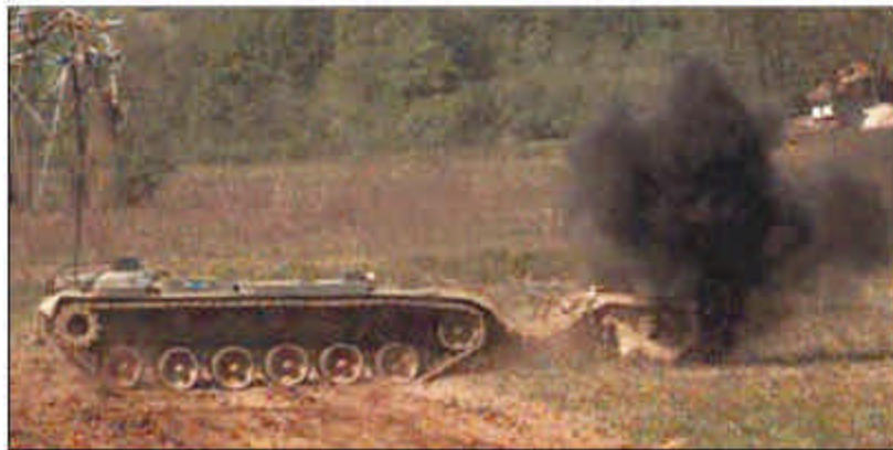
Figure 2-5: Teleoperated turretless M-60 Panther detonating anti-personnel mine in Bosnia [6]
