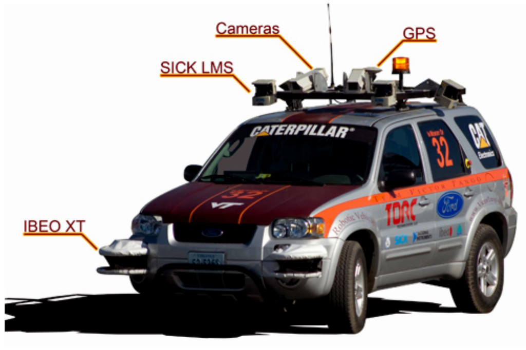
Figure 2.2: Odin's external sensor suite provided the software with valuable obstacle and positioning data during the 2007 Urban Challenge.
