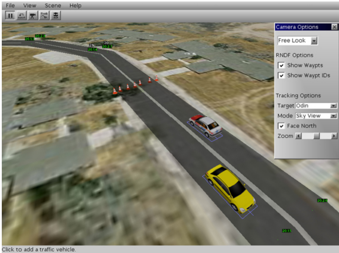
Figure 6.2: Static obstacles, traffic, and RNDFs can be displayed over aerial imagery in Team Victor Tango's simulator [18].
