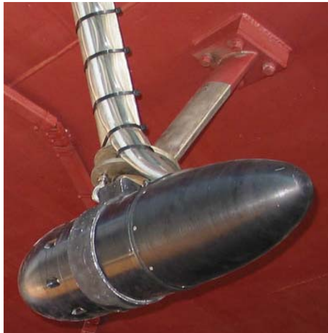
Figure 12 – Installed PIV Camera
