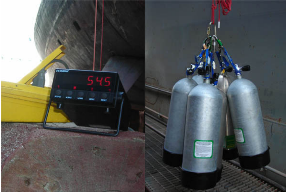
Figure 9 – Calibration Setup Load cell output shown on the left, weights on the right.
