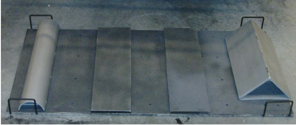
Figure 3-15: Sample Surface for Transverse and Longitudinal Calibration
