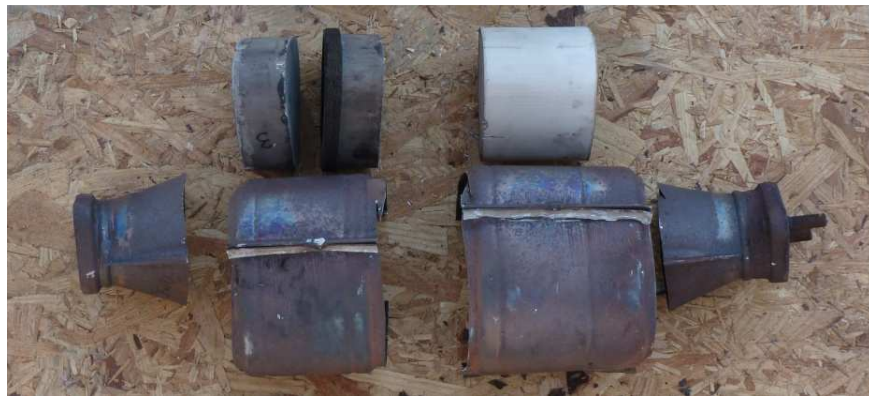
Figure 2.1: Cut-apart catalytic converter. (Photo by author, 2012).
