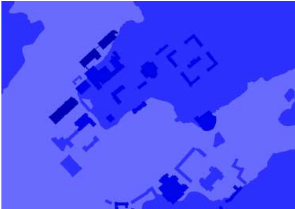
Figure 3.3 DEM showing flat rooftop elevations
