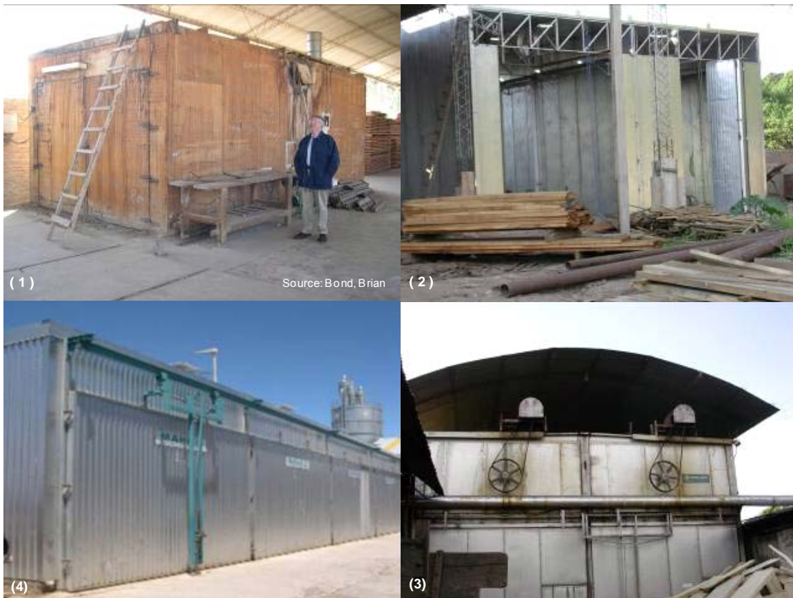
Figure 2-8. Examples of kiln technology: (1) wooden kiln, (2) kiln in construction, (3) 27-year-old line-shaft Irvington Moore kiln and, (4) automatic-controlled Mahil kilns.
