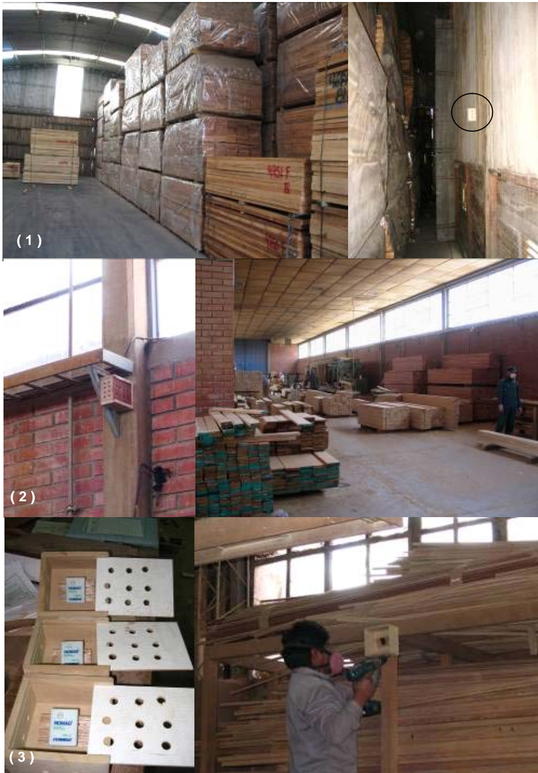
Figure 4-6. Location of temperature and humidity sensors in: (1) storage facilities in Santa Cruz, (2) flooring and furniture parts plant in La Paz, and (3) protective boxes and door plant in Cochabamba.
