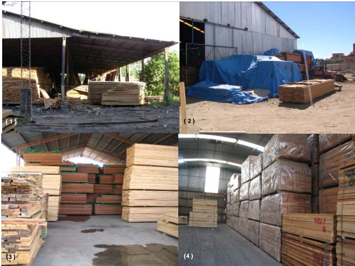
Figure 3-7. Storage of dry lumber: (1) shed with un-surfaced soil, (2) outdoor storage of tarp-covered lumber, (3) open shed storage, (4) plastic-wrapped packs of dry lumber.
