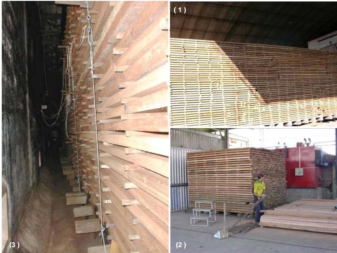
Figure 3-4. Lumber stacking practices in Bolivia: (1) stacking different lumber lengths in a truck-kiln pile, (2) all stacking is made by hand, (3) using cables and turnbuckles to restrain the top layers of lumber.
