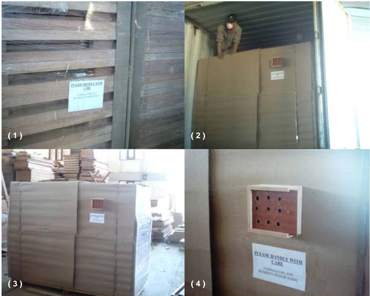
Figure 4-7. Data logger placement for solid doors shipping study: (1) sensor inside package, (2) doors package inside container, (3) door pallet ready for shipment, and (4) outside sensor's in protective box.
