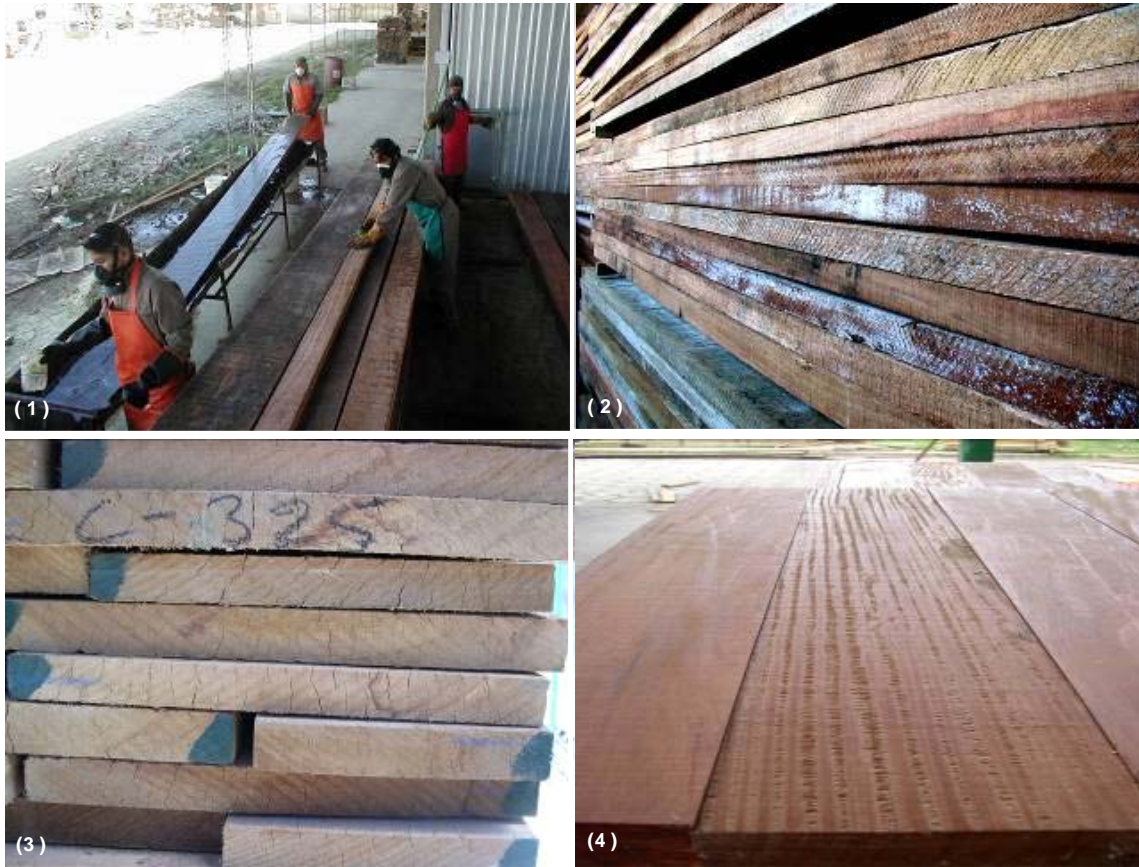
Figure 3-6. Drying defects: (1) manual dip-soaking lumber, (2) mold and fungal stain in dried Bibosi ( Ficus glabrata ), (3) extensive end-checking in Almedrillo, (4) tension wood in Paquió.
