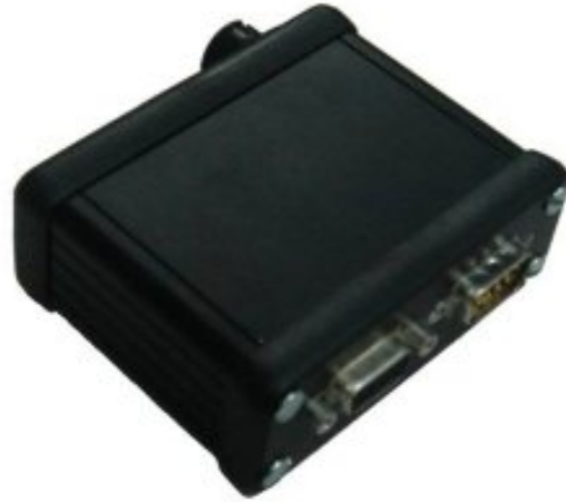
Figure 2.9: Relay Interface Board inside enclosure.
