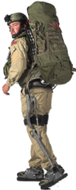
Figure 2.3 The ExoHiker™ attached to an individual. It is designed to carry a heavy load in the backpack portion of the exoskeleton. This is a good example of how small and sleek exoskeletons have become. [Berkeley Bionics (2008)]
