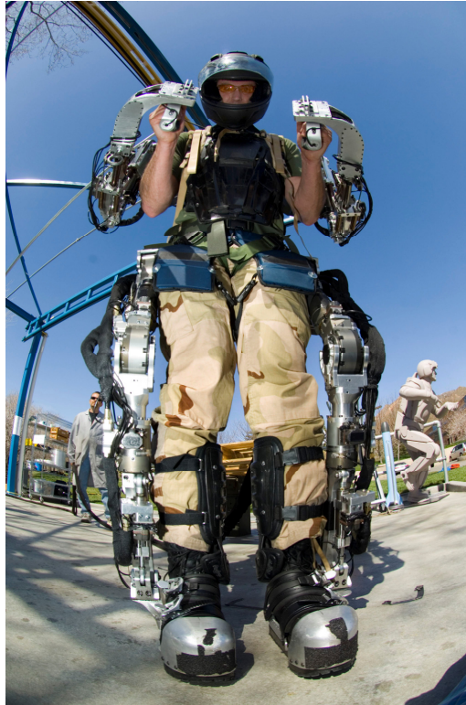
Figure 2.4 The full body XOS exoskeleton. This recently publicized hydraulic powered exoskeleton is probably the most capable exoskeleton to date. However, it is currently tethered for power reasons. [© Raytheon (2008)]
