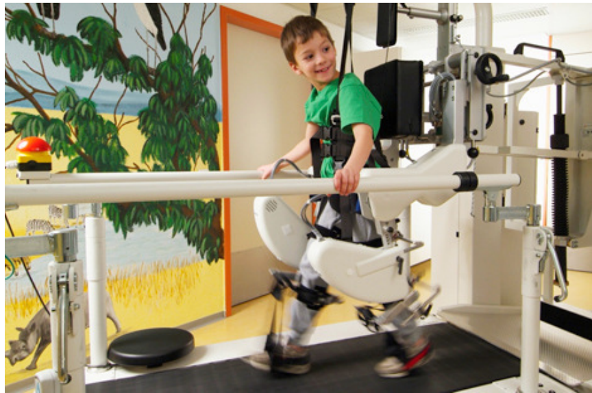
Figure 2.1 The pediatric Lokomat. It is shown moving a child's legs through the motions of walking on the treadmill below foot. The pediatric version is similar to the Lokomat for adults, but contains a smaller harness, cuffs, and extremity attachments to fit a child. The programmed gait motions are also altered for a child's movements. ©Hocoma AG, Switzerland, www.hocoma.com [Hocoma (2008)]
