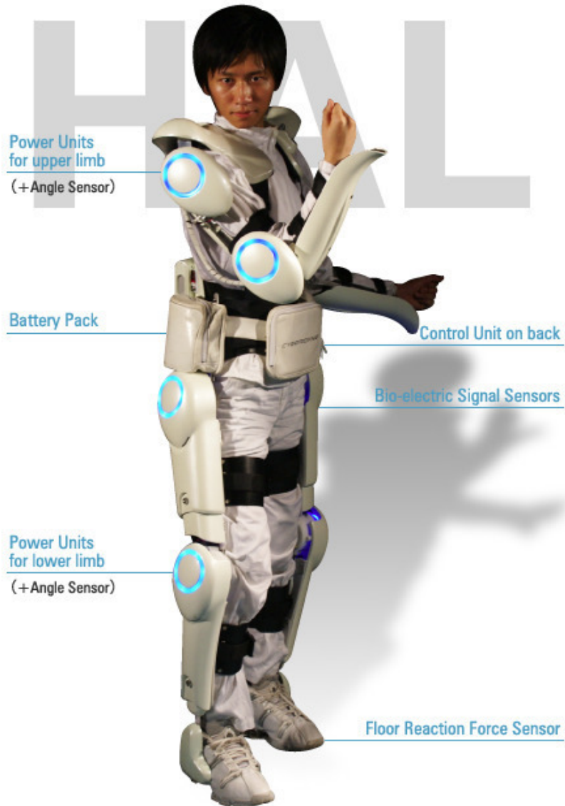
Figure 2.5 The HAL-5 exoskeleton. The connection points, motor, power, and computing component locations are labeled. Special attention should be paid tot the physical connections on the torso, upper legs, lower legs, and the feet. [Cyberdyne, Inc. (2008), Prof. Sankai, University of Tsukuba]
