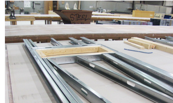
Figure 3.4.1.1: Steel frame wall panels are fitted with 2x4 wood construction for easy window/door installation.
