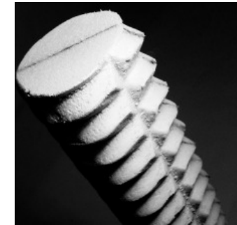
Figure 2.5.3 CNC-milled 4x4: Object created by a 3-axis CNC router, using the surfaces modeled in Rhino to define the toolpath boundaries in MasterCAM.
