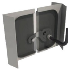
Figure A.4 cam lock mechanism
