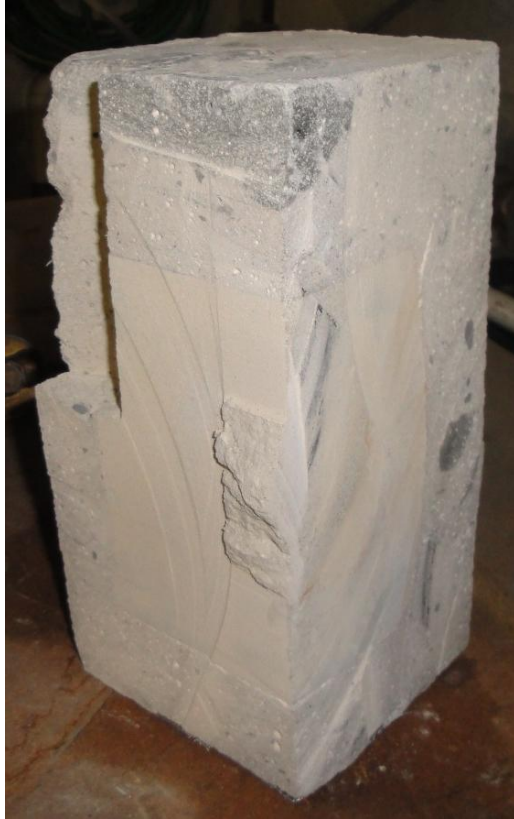
Figure B-13: Caprock sample from test number one, post testing cut into quarters. With injection tube at the bottom, bottom right quadrant is displayed.
