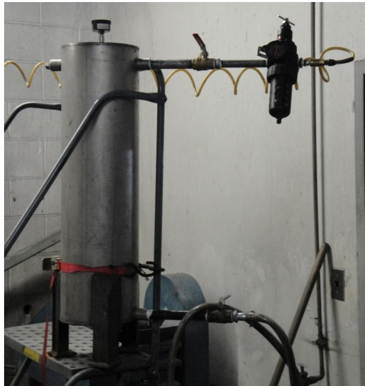
Figure B-7: Schematic Pressure tank with injection tube and air regulator.
