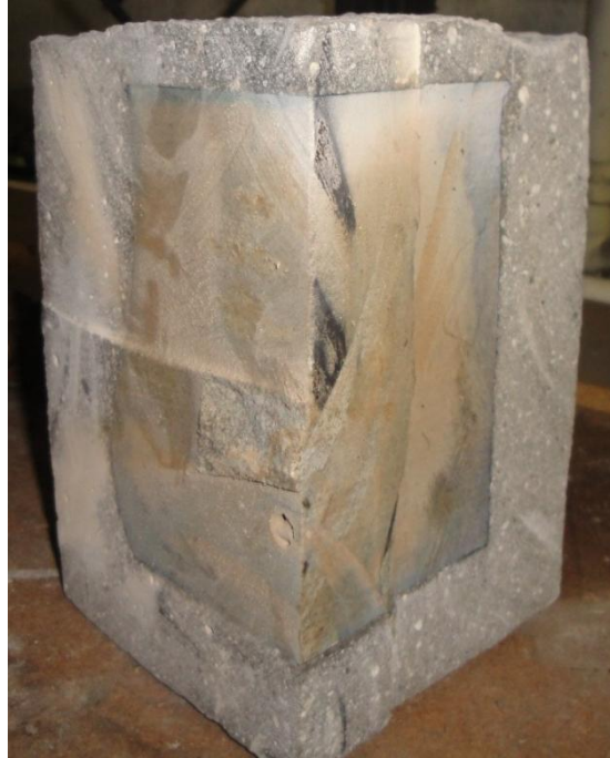
Figure B-27: Caprock sample from test number five, post testing cut into quarters. With injection tube at the bottom, top left quadrant is displayed.
