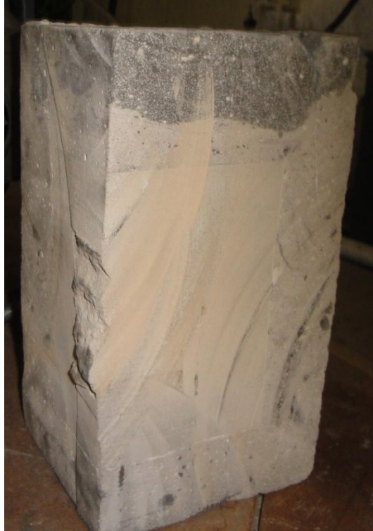
Figure B-11: Caprock sample from test number one, post testing cut into quarters. With injection tube at the bottom, top left quadrant is displayed.
