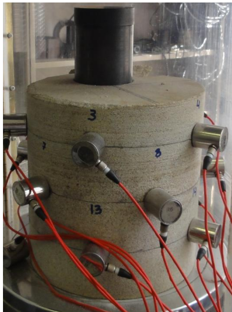
Figure 3.6: A prepared sample of Berea Sandstone with sensors attached and indenter in desired location
