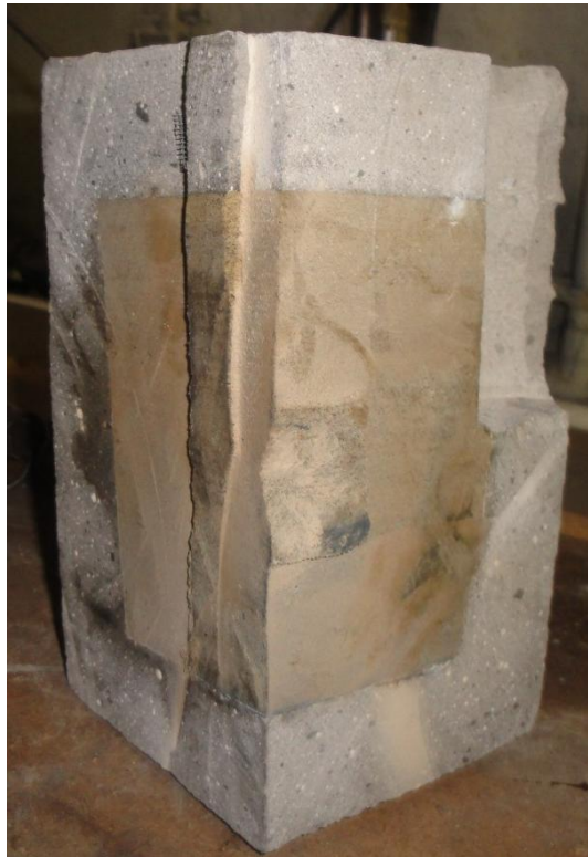
Figure B-20: Caprock sample from test number three, post testing cut into quarters. With injection tube at the bottom, top right quadrant is displayed.
