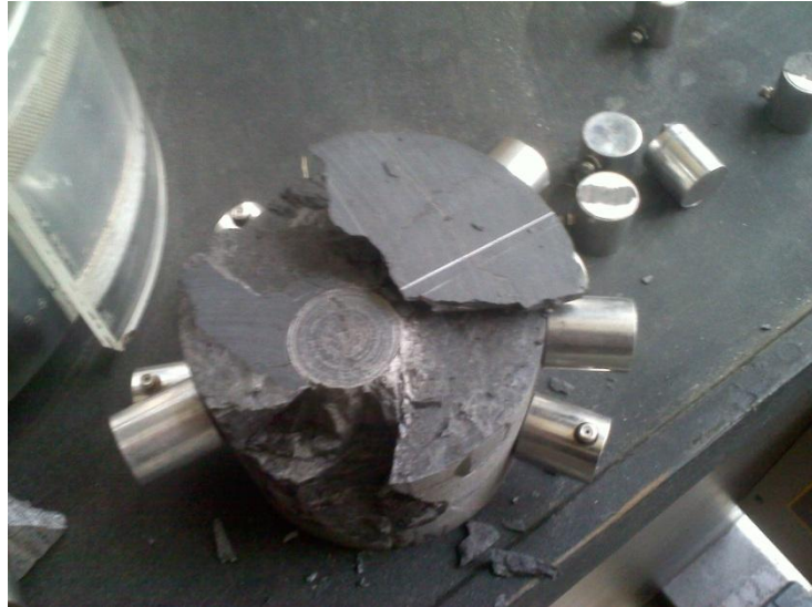
Figure 3.30: Failed sample of Marcellus Shale after indenter test was concluded.
