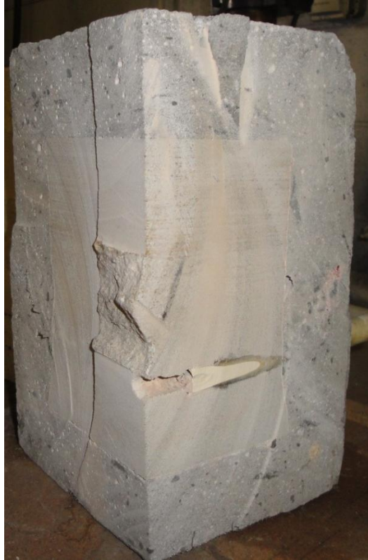
Figure B-17: Caprock sample from test number two, post testing cut into quarters. With injection tube at the bottom, bottom right quadrant is displayed.
