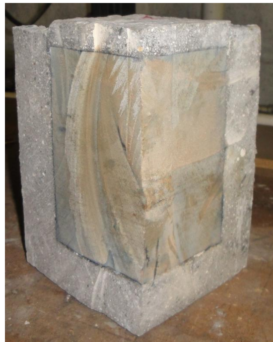
Figure B-28: Caprock sample from test number five, post testing cut into quarters. With injection tube at the bottom, top right quadrant is displayed.
