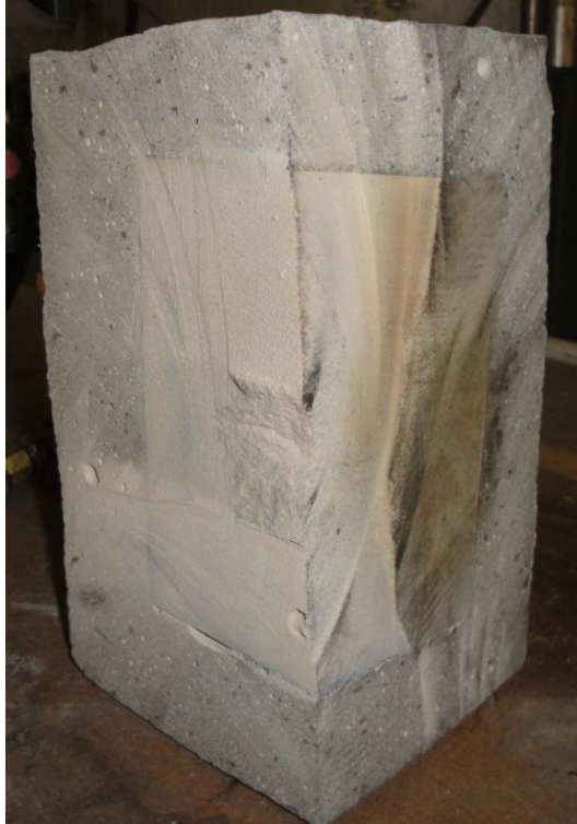
Figure B-19: Caprock sample from test number three, post testing cut into quarters. With injection tube at the bottom, top left quadrant is displayed.
