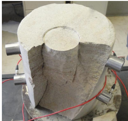
Figure 3.19: Failed sample of Berea Sandstone after indenter test was concluded.
