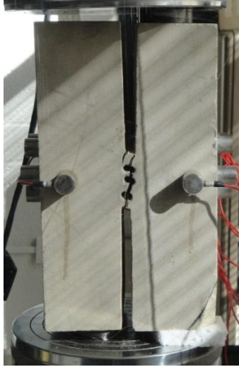
Figure 4.2: Failed shear test sample.
