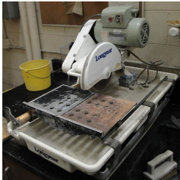
Figure A-3: Stone saw used to prepare core samples.
