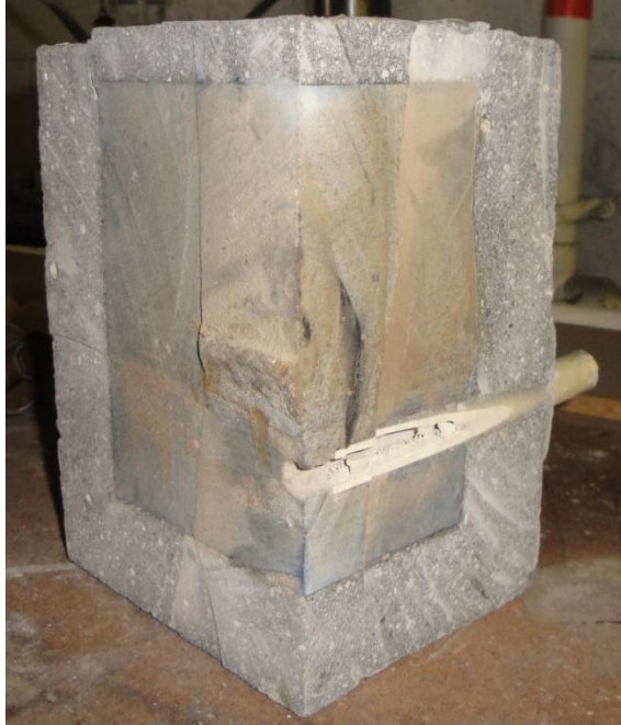
Figure B-29: Caprock sample from test number five, post testing cut into quarters. With injection tube at the bottom, bottom right quadrant is displayed.
