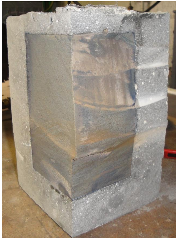
Figure B-34: Caprock sample from test number six, post testing cut into quarters. With injection tube at the bottom, bottom left quadrant is displayed.
