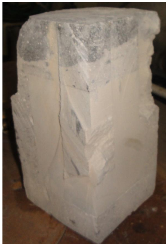
Figure B-12: Caprock sample from test number one, post testing cut into quarters. With injection tube at the bottom, top right quadrant is displayed.
