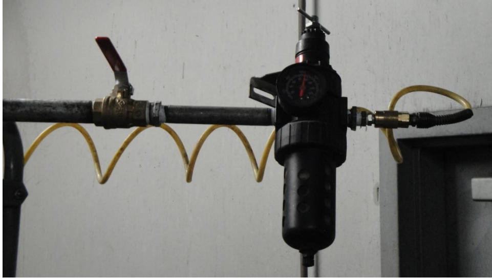
Figure B-8: Air regulator and air cutoff valve for fluid pressure tank.
