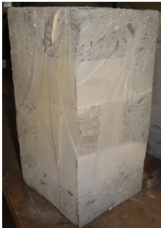
Figure B-18: Caprock sample from test number two, post testing cut into quarters. With injection tube at the bottom, bottom left quadrant is displayed.
