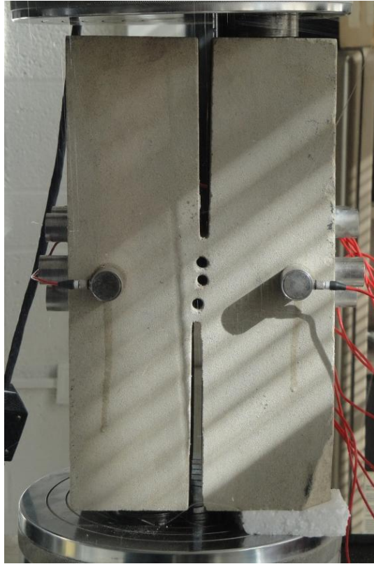
Figure B-2: Berea Sandstone shear sample prior to failure.
