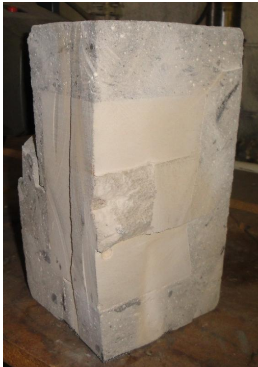
Figure B-16: Caprock sample from test number two, post testing cut into quarters. With injection tube at the bottom, top right quadrant is displayed.
