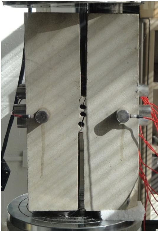
Figure B.3: Berea Sandstone shear sample post failure.
