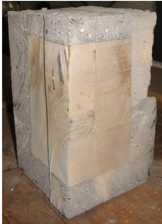
Figure B-24: Caprock sample from test number four, post testing cut into quarters. With injection tube at the bottom, top right quadrant is displayed.
