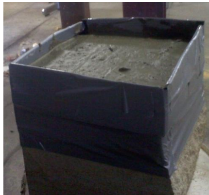
Figure 4.5: Form made of rubber for fifth and sixth sample to pour caprock first.
