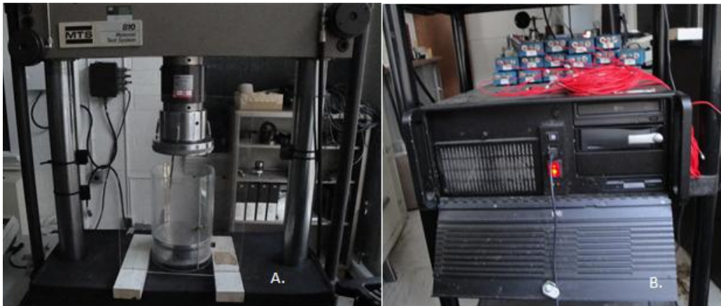
Figure 3.7: Side A is the MTS 810 Material Test System. Side B is the ESG Solutions Hyperion system.
