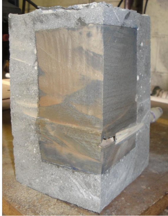
Figure B-33: Caprock sample from test number six, post testing cut into quarters. With injection tube at the bottom, bottom right quadrant is displayed.
