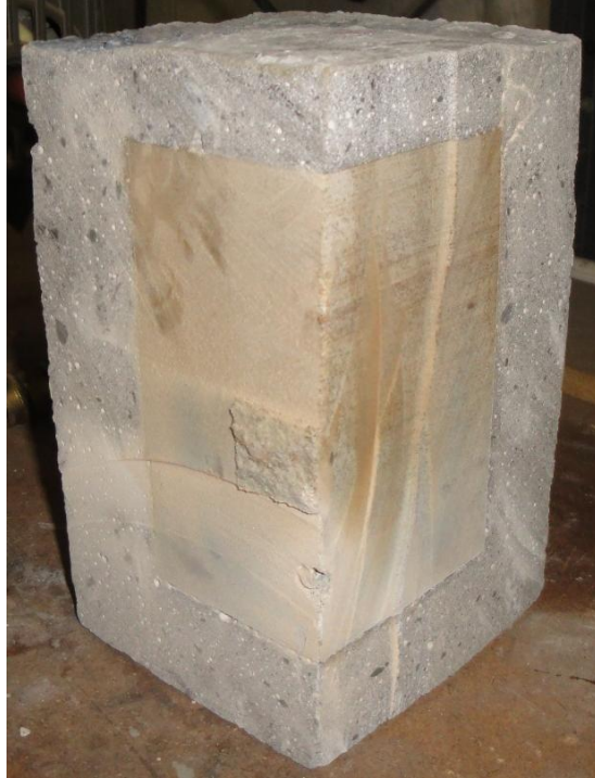
Figure B-23: Caprock sample from test number four, post testing cut into quarters. With injection tube at the bottom, top left quadrant is displayed.
