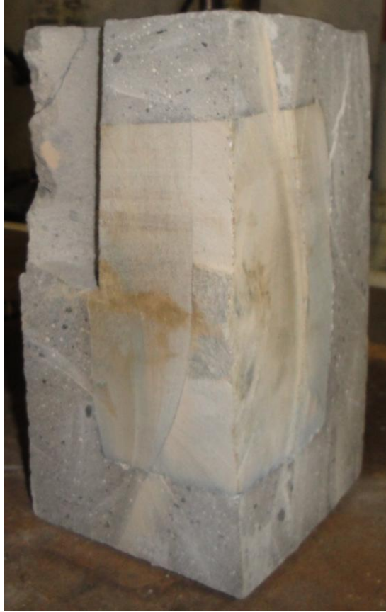
Figure B-21: Caprock sample from test number three, post testing cut into quarters. With injection tube at the bottom, bottom right quadrant is displayed.
