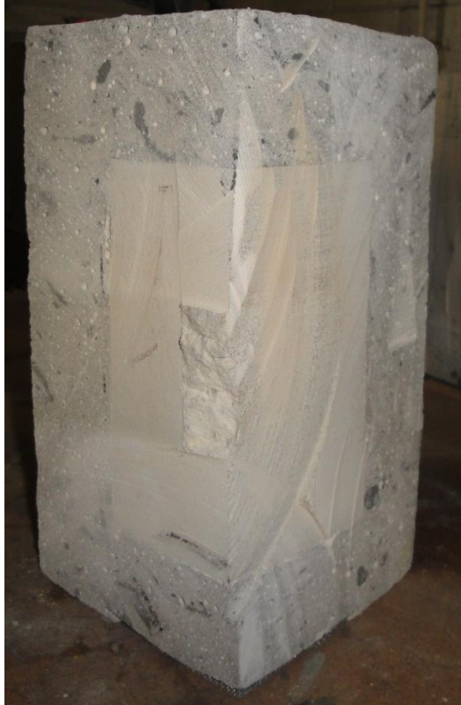
Figure B-15: Caprock sample from test number two, post testing cut into quarters. With injection tube at the bottom, top left quadrant is displayed.
