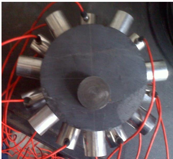
Figure A-6: Top view of the Marcellus Shale sample prior to testing.
