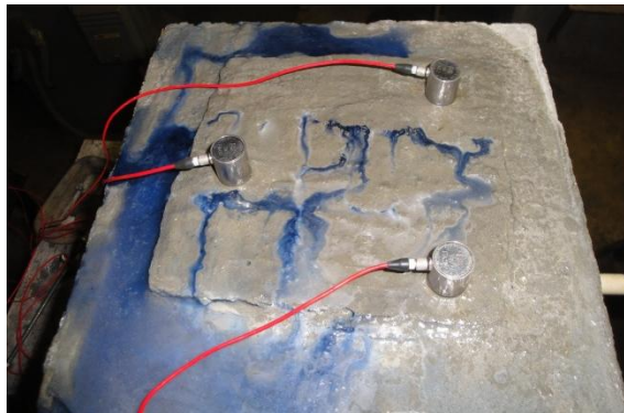
Figure 4.7: Dyed fluid escaping through artificial fault in a caprock sample.
