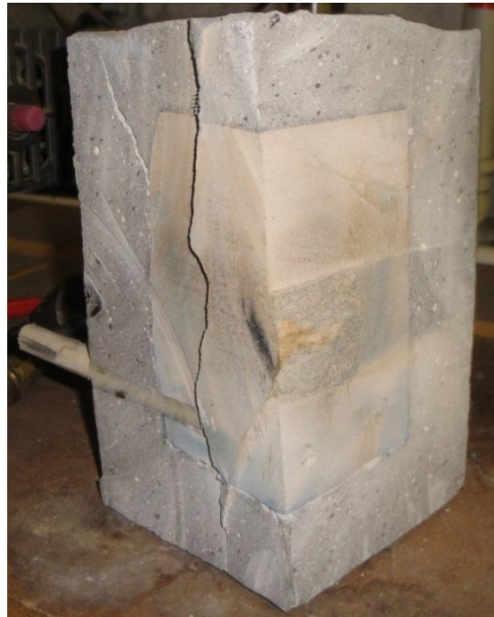
Figure B-22: Caprock sample from test number three, post testing cut into quarters. With injection tube at the bottom, bottom left quadrant is displayed.
