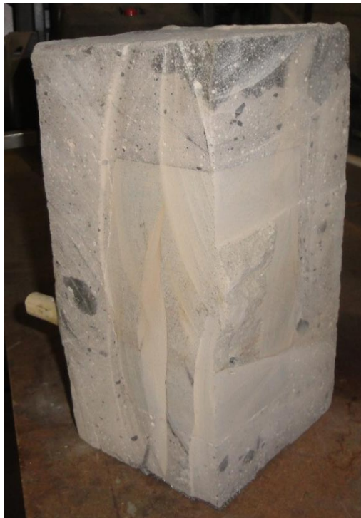
Figure B-14: Caprock sample from test number one, post testing cut into quarters. With injection tube at the bottom, bottom left quadrant is displayed.
