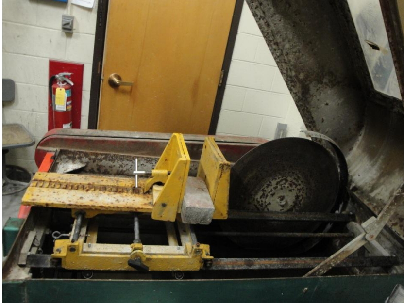
Figure A-4: Stone saw with 8 inch blade used to cut Marcellus Shale and Berea Sandstone samples.
