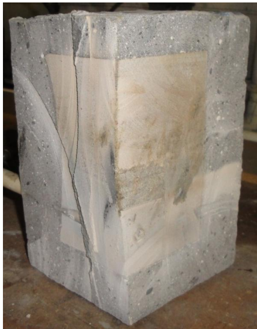
Figure B-26: Caprock sample from test number four, post testing cut into quarters. With injection tube at the bottom, bottom left quadrant is displayed.
