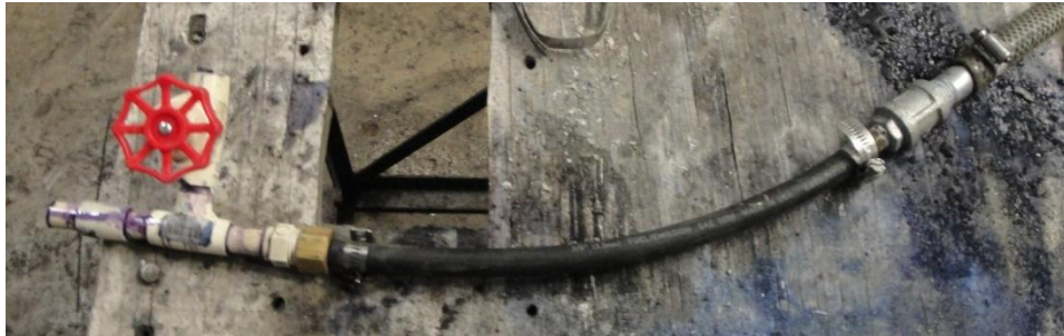
Figure B-9: Fluid injection tube with air bleeder valve.
