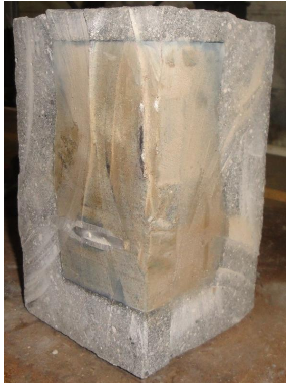
Figure B-30: Caprock sample from test number five, post testing cut into quarters. With injection tube at the bottom, bottom left quadrant is displayed.
