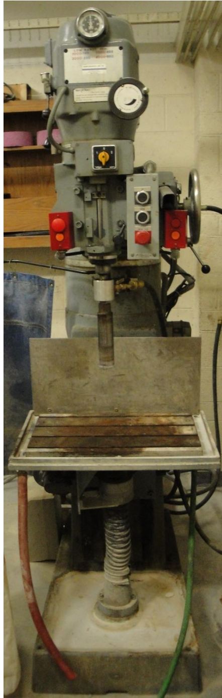
Figure A-1: Stone drill press used to cut Berea Sandstone samples
