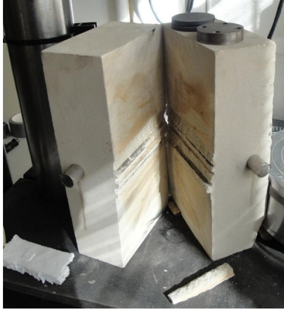
Figure B-4: Berea Sandstone shear sample after halves were separated post failure.
