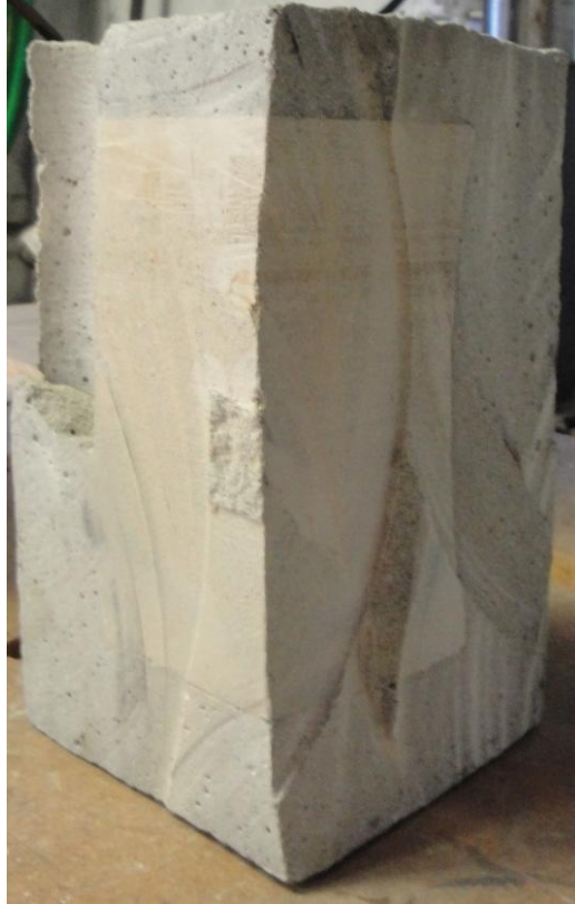
Figure B-25: Caprock sample from test number four, post testing cut into quarters. With injection tube at the bottom, bottom right quadrant is displayed.
