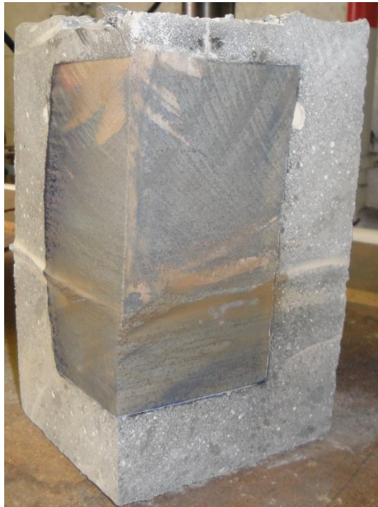
Figure B-32: Caprock sample from test number six, post testing cut into quarters. With injection tube at the bottom, top right quadrant is displayed.
