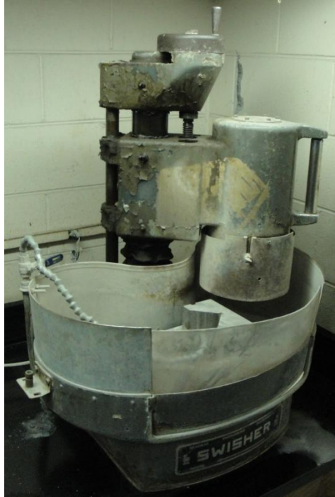
Figure A-2: Stone grinder, used to smooth the faces of the Marcellus Shale sample.
