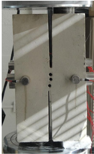
Figure 4.1: Shear failure test with sensors attached
