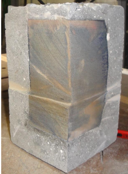
Figure B-31: Caprock sample from test number six, post testing cut into quarters. With injection tube at the bottom, top left quadrant is displayed.
