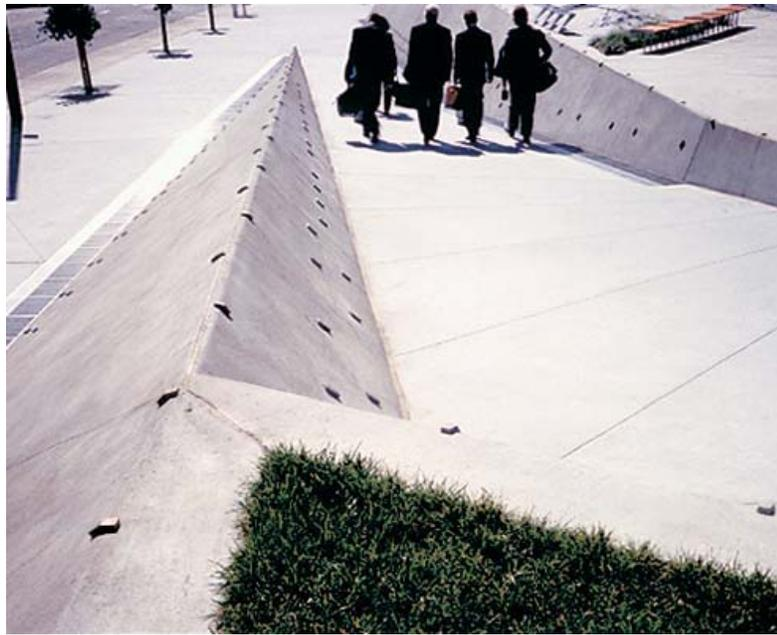
Figure 21, Berms as Vehicle Barriers, Phillip Burton Federal Building and U.S. Courthouse, San Francisco, California
