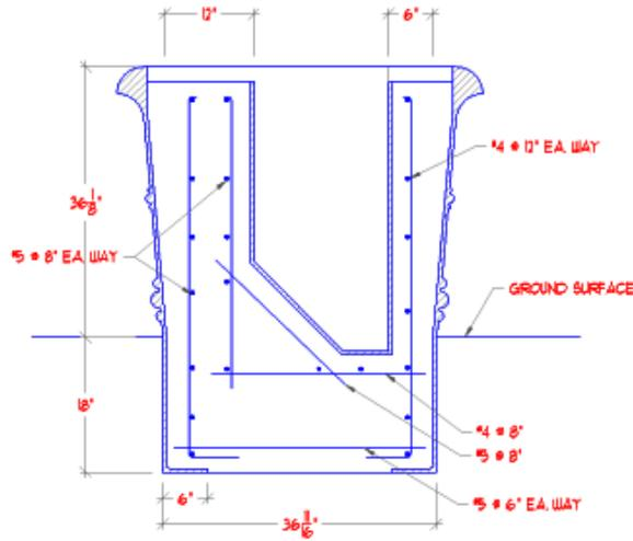
Figure 16, Planter Box Cross Section
