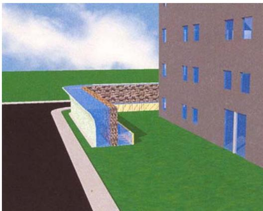
Figure 24, Combination Barrier, Composed of a Wall of Water and a Reinforced Concrete Wall
