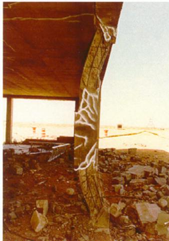
*Ductile and nearly elastic response to same blast after wrapped with fiber reinforced polymer (FRP)*
