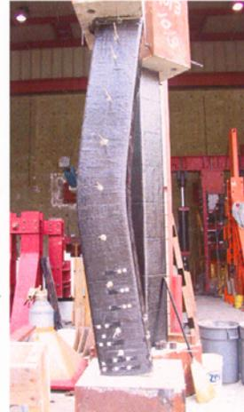
Figure 28, Column Blast Tests
