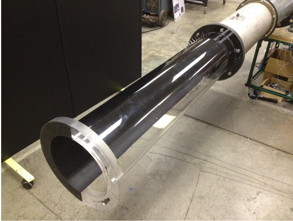
Figure 2.6. Can combustor model used with PIV measurements (Photo by Author)
