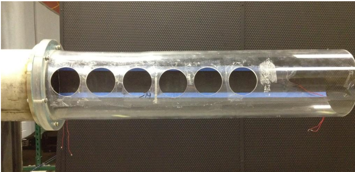
Figure 2.5. Can combustor model with viewports used for heat transfer measurements (Photo by Author)
