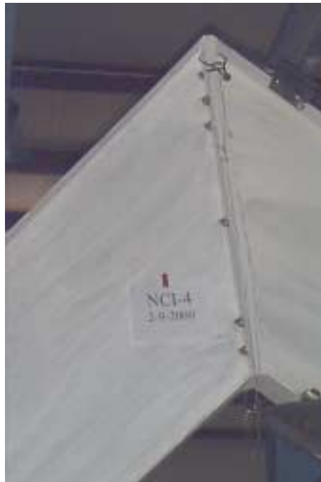
b) Connection Subsequent to Testing (Note: No significant yielding or plate separation is visible.)
