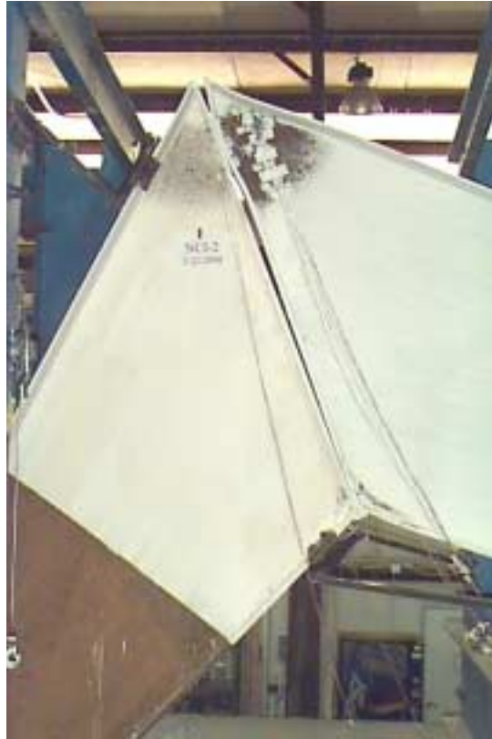
a) Yielding of Column and Rafter End-Plate
