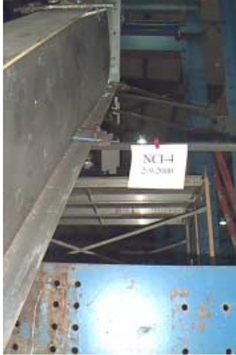
a) Web Buckling of Column (near connection)
