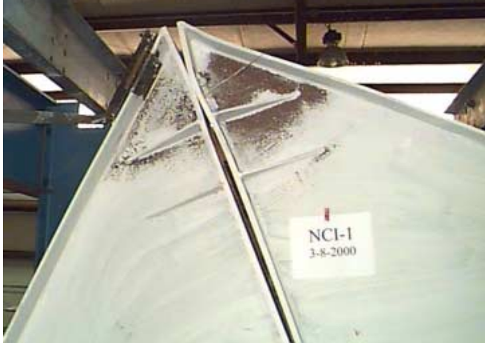
a) Yielding of Column and Rafter Web
