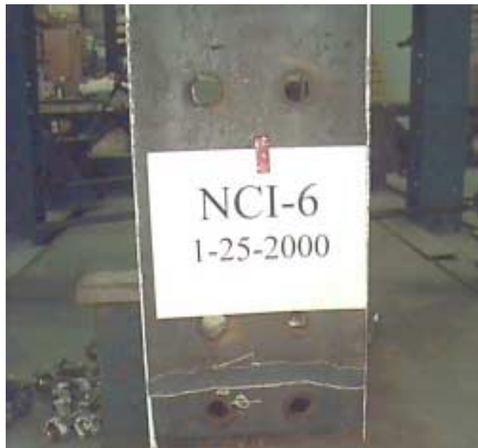
d) Yielding of End-Plate (Note: Chalk was used to outline where yielding has occurred.)
