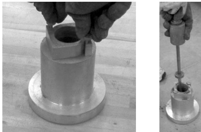
Figure 3. Cylinder Mold Stand (left) and Special Hammer (right)
