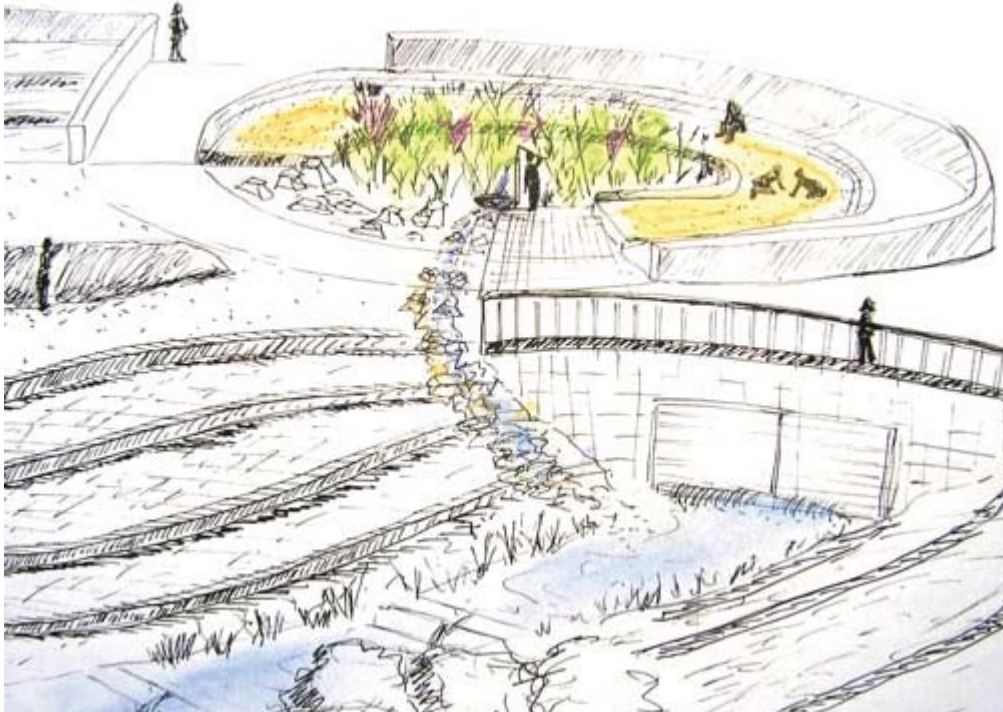
Sketch showing Interactive Rain Garden and dry river bed transporting purified stormwater runoff into the stream.
