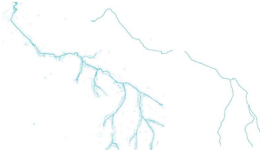
Figure 5. Form of Watts Branch Before and After Channelization
