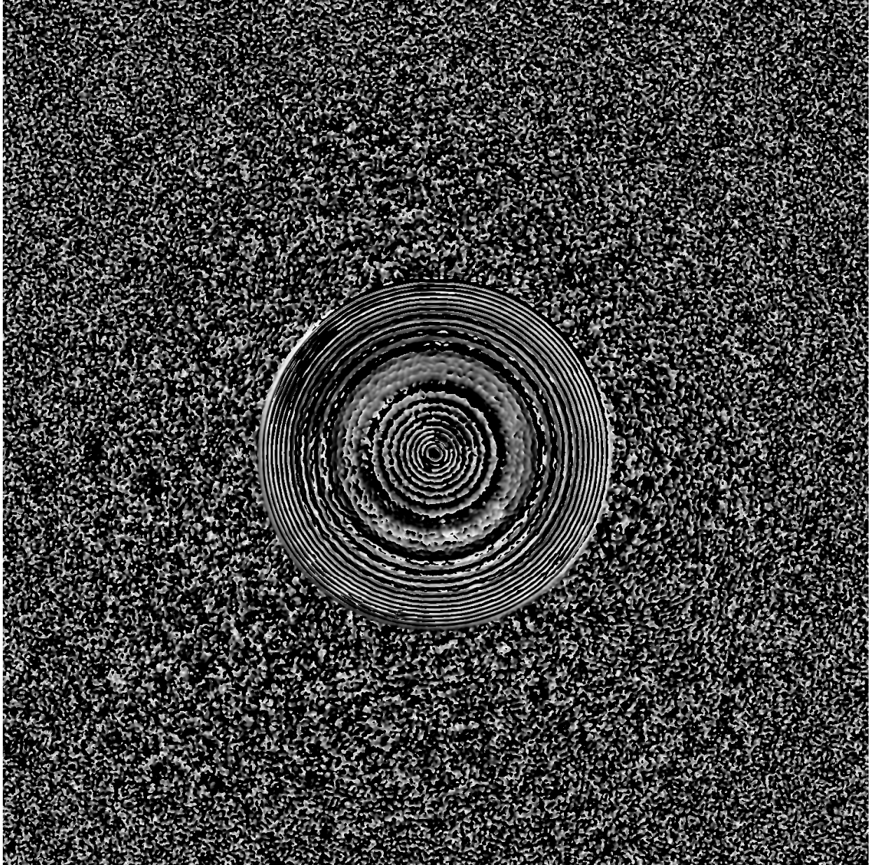
Figure 3-3(b) Phase plot: Reconstruction of the pinhole hologram 131207_11 at depth z = 85 \mu m using only mathematical \mathfrak{H}(k_x, k_y; z_R) .
