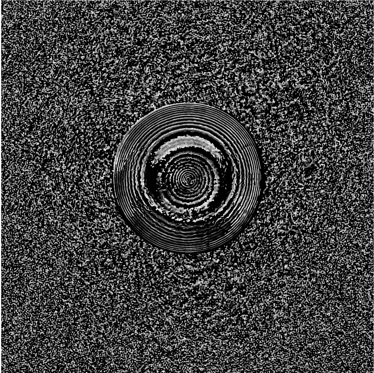
Figure 3-2(b) Phase plot: Reconstruction of the pinhole hologram 131207_11 with the pinhole hologram 131207_19 propagated to depth z = 85 \mu\text{m} .
