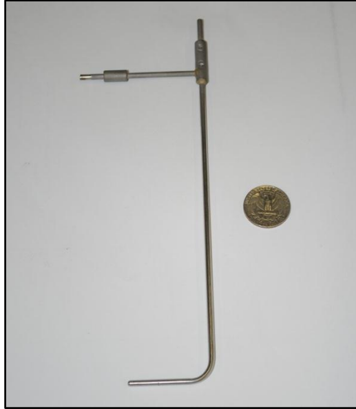
FIGURE 4.6. PITOT-STATIC TUBE SHOWING SCALE
