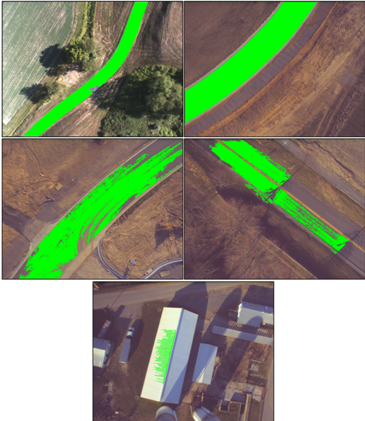
Figure 6.8: Examples of results from roadway detection algorithm on different types of images: (Top Left) Type I, (Top Right) Type II, (Middle Left) Type III, (Middle Right) Type IV, (Bottom Middle) Type V
