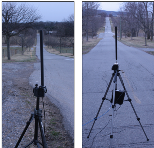
Figure 4.3: Setup of antennas for the radiation pattern experiment - 434 meters between antennas
