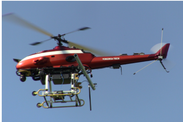
Figure 5.3: RMAX unmanned helicopter used in radio repeating test ( Image courtesy of Matt Torok, USL Graduate Student )
