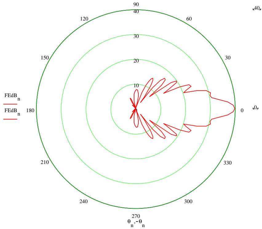
Figure A.5 Downlink Horn Perimeter Beam, Total Pattern in YZ plane (*E*-plane)
