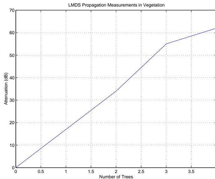
Figure 6.2 Vegetation Losses as a function of Number of Trees in the Propagation Path
