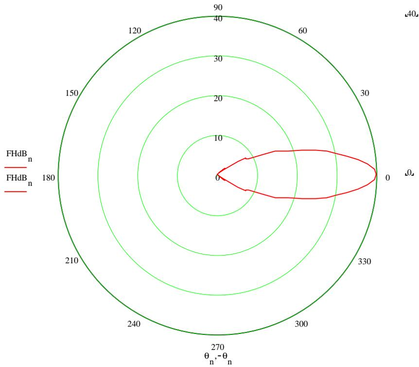
Figure A.6 Downlink Horn Perimeter Beam, Total Pattern in XZ plane (*H*-plane)
