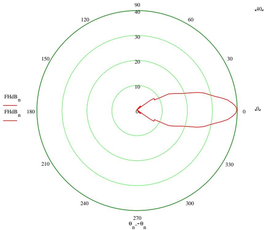
Figure A.8 Uplink Horn, Total Pattern in XZ plane ( $H$ -plane)
