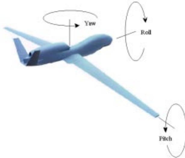
Figure 5.5 Roll, Pitch and Yaw Illustration
