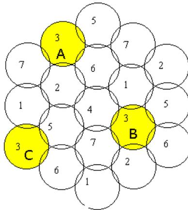
Figure 6.1 UAV-LMDS Frequency Reuse Pattern and Interfering Beams
