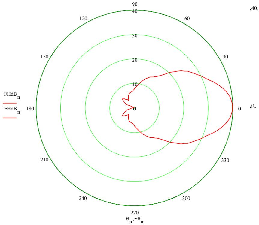
Figure A.4 Downlink Horn Middle Beam, Total Pattern in XZ plane (*H*-plane)
