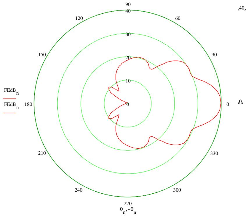
Figure A.3 Downlink Horn Middle Beam, Total Pattern in YZ plane (*E*-plane)
