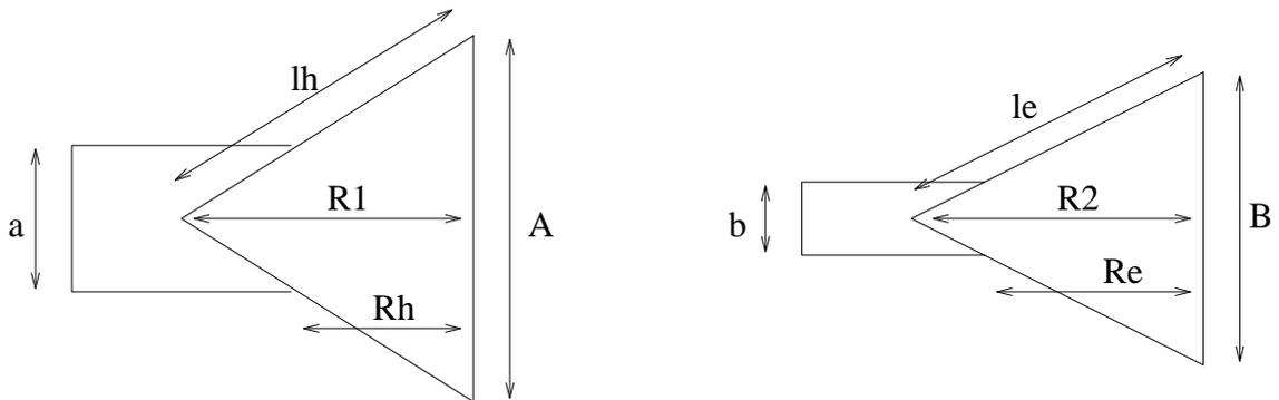
Figure 3.2 Pyramidal Horn Diagram
