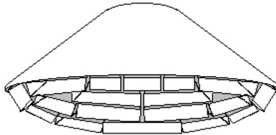
Figure 5.4 Pyramidal Horn Arrangement
