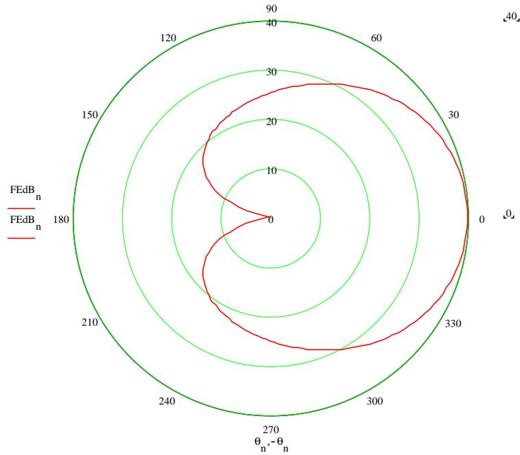
Figure A.1 Downlink Horn Center Beam, Total Pattern in YZ plane ( $E$ -plane)
