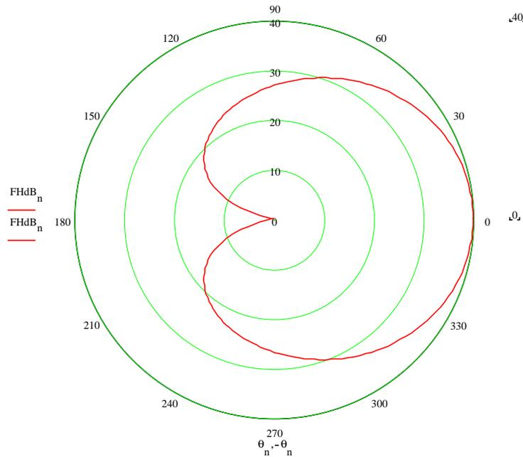
Figure A.2 Downlink Horn Center Beam, Total Pattern in XZ plane ( $H$ -plane)
