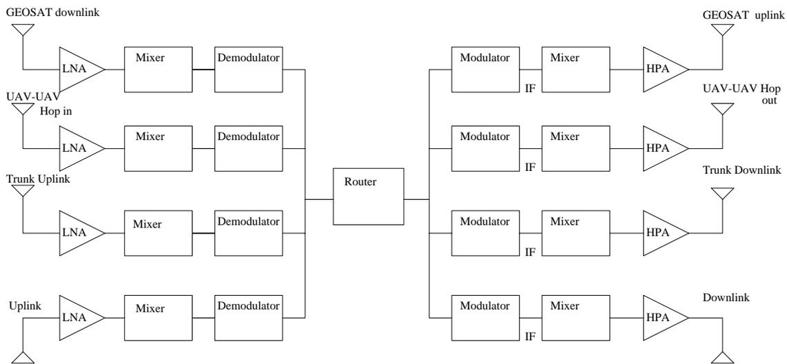
Figure 5.7 Global Hawk Communication Payload
