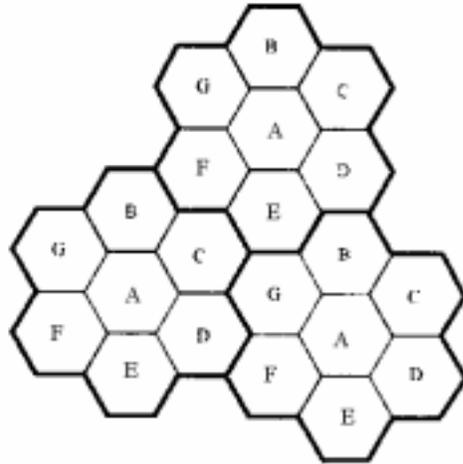
Figure 3.3 Cellular Frequency Reuse Pattern
