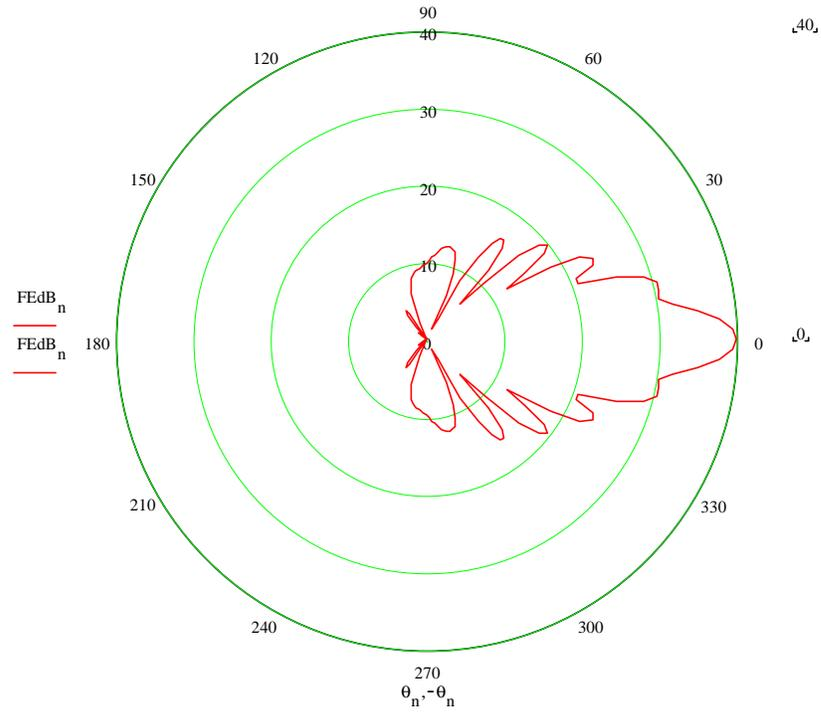
Figure A.7 Uplink Horn, Total Pattern in YZ plane ( $E$ -plane)
