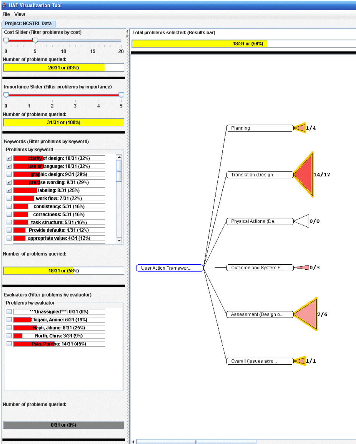
Figure 42: The results bar at the top of the screen show 18/31 or 58% of the usability problems deal with the keywords checked on left side (Keyword area). The keywords checked all deal with wording. This insight gives the user the ability to improve the process rather than just the individual usability problems.
