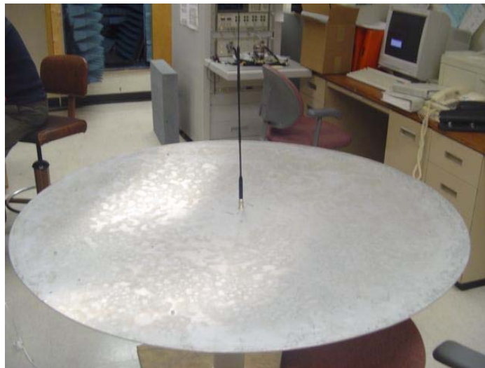
Figure 5-4 3 rd Measurement: 50-1200 MHz; Circular Ground Plane
