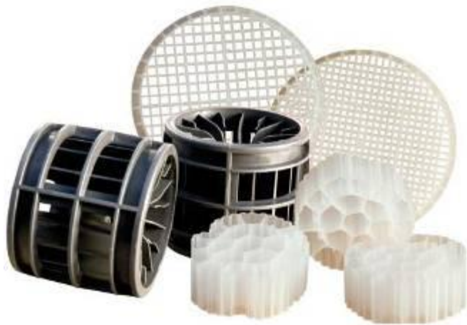
Figure 2.1 AnoxKaldnes TM BiofilmChip TM P ( \sim 900 \text{ m}^2/\text{m}^3 ), BiofilmChip TM M ( \sim 1200 \text{ m}^2/\text{m}^3 ), F3 ( \sim 220 \text{ m}^2/\text{m}^3 ), and K3 ( \sim 500 \text{ m}^2/\text{m}^3 )
