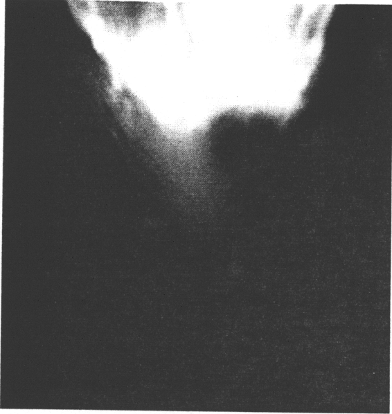
Figure 3.6: Burning carbon dioxide-atomized spray (momentum controlled).
