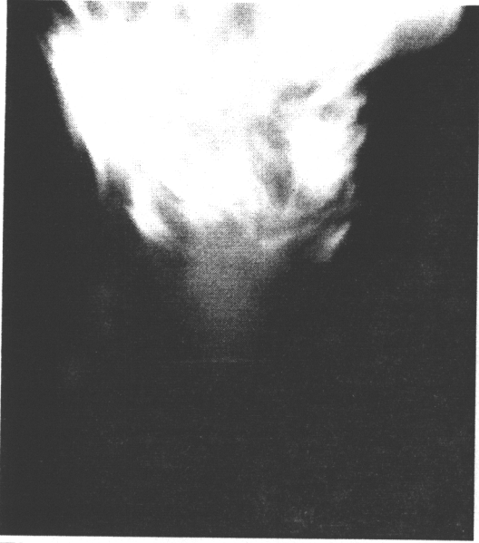
Figure 3.5: Burning argon-atomized spray (momentum controlled).
