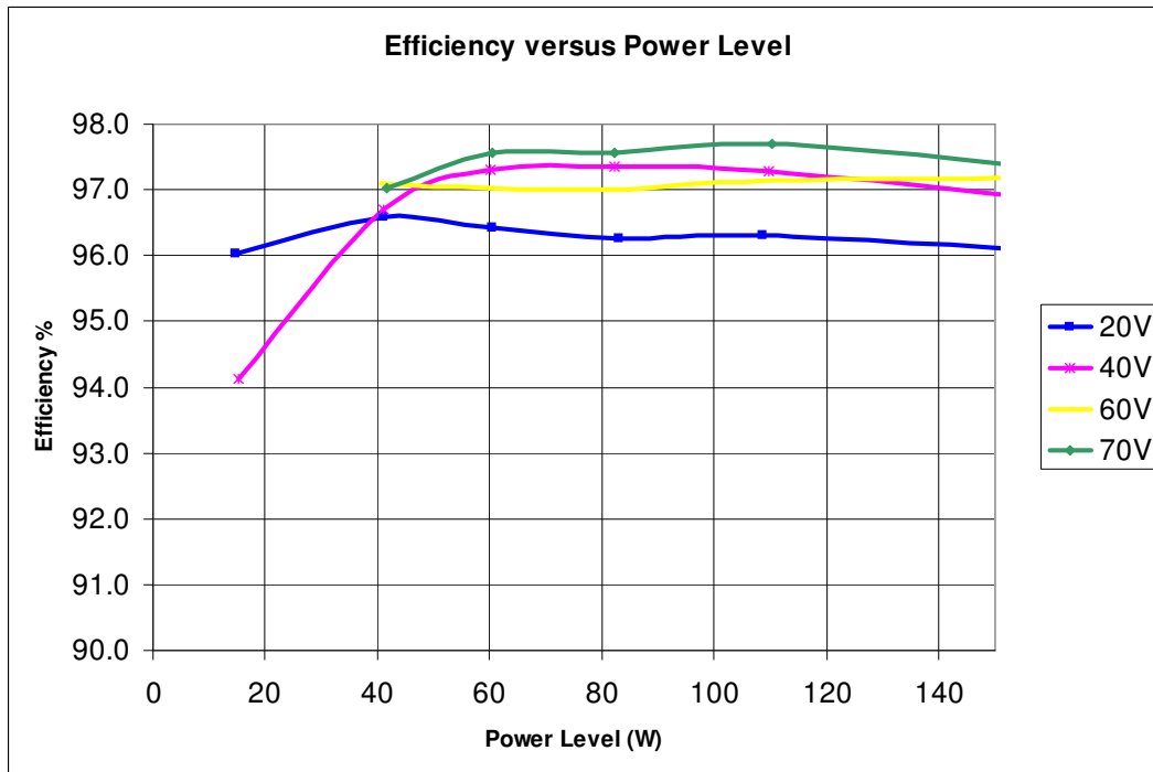
Figure 26. DC-DC Efficiency with Oversized Components
