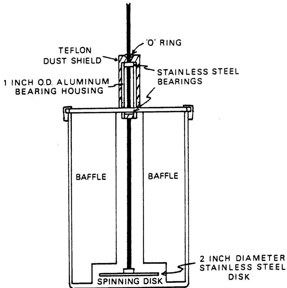
Figure 2.9 The microbubble dispersion generator (Kaster, 1988).
