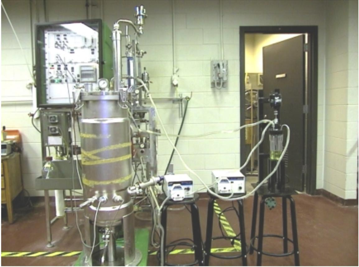
Figure 3.2 50-liter fermentation with microbubble dispersion unit.
