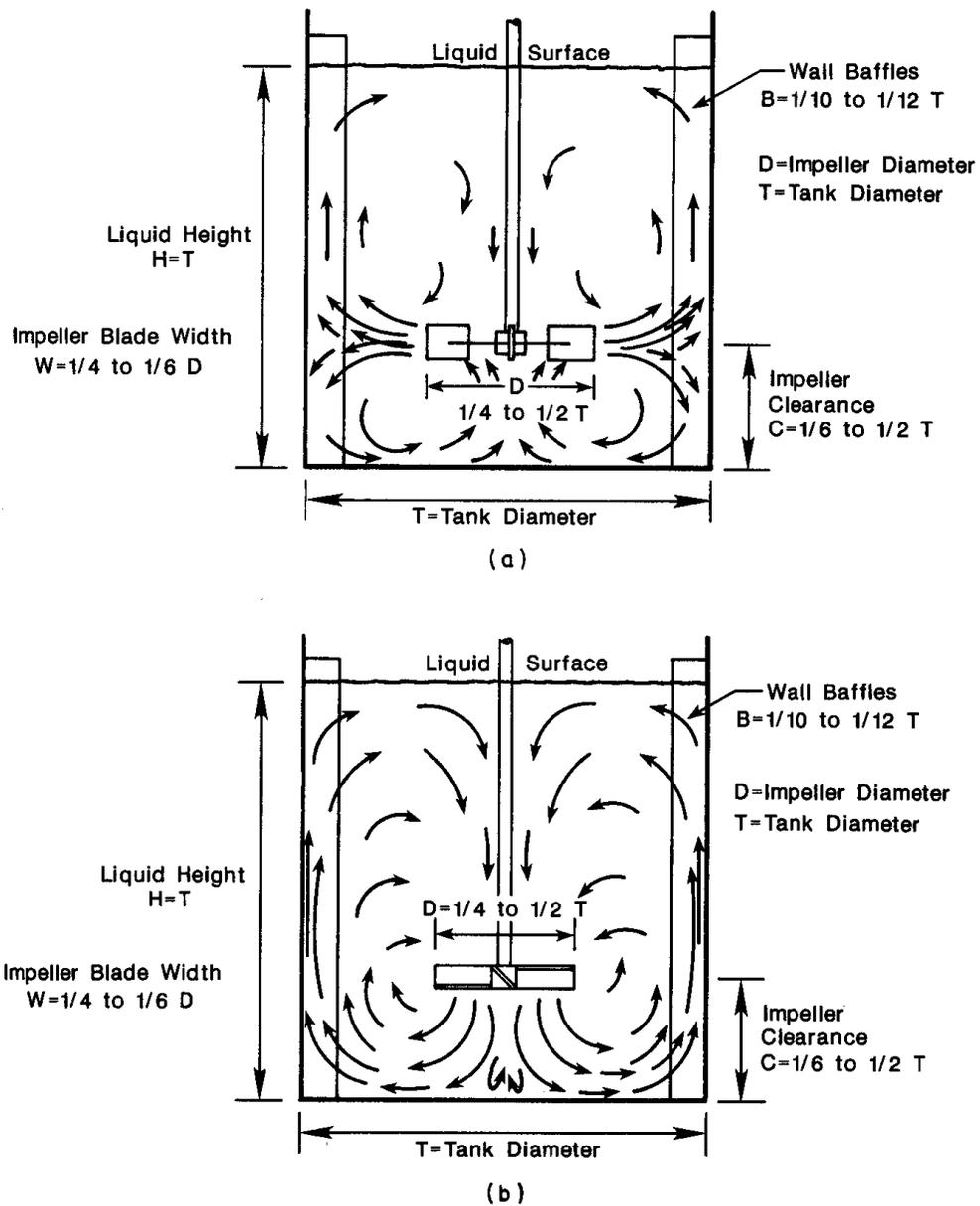
Figure 2.10 The standard geometry of mixing tank (Tatterson, 1991).
