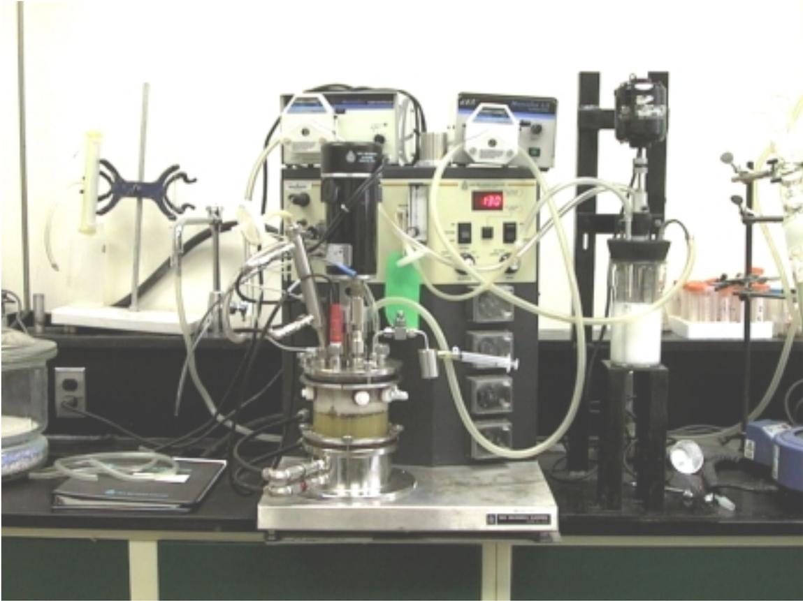
Figure 3.1 1-liter fermentation with microbubble dispersion unit
