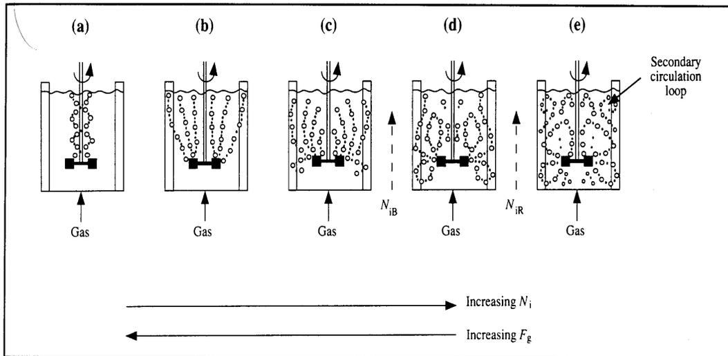
**Figure 2.2 Different patterns of gas bubble dispersion in a stirred-tank reactor (Doran, 1995).**
