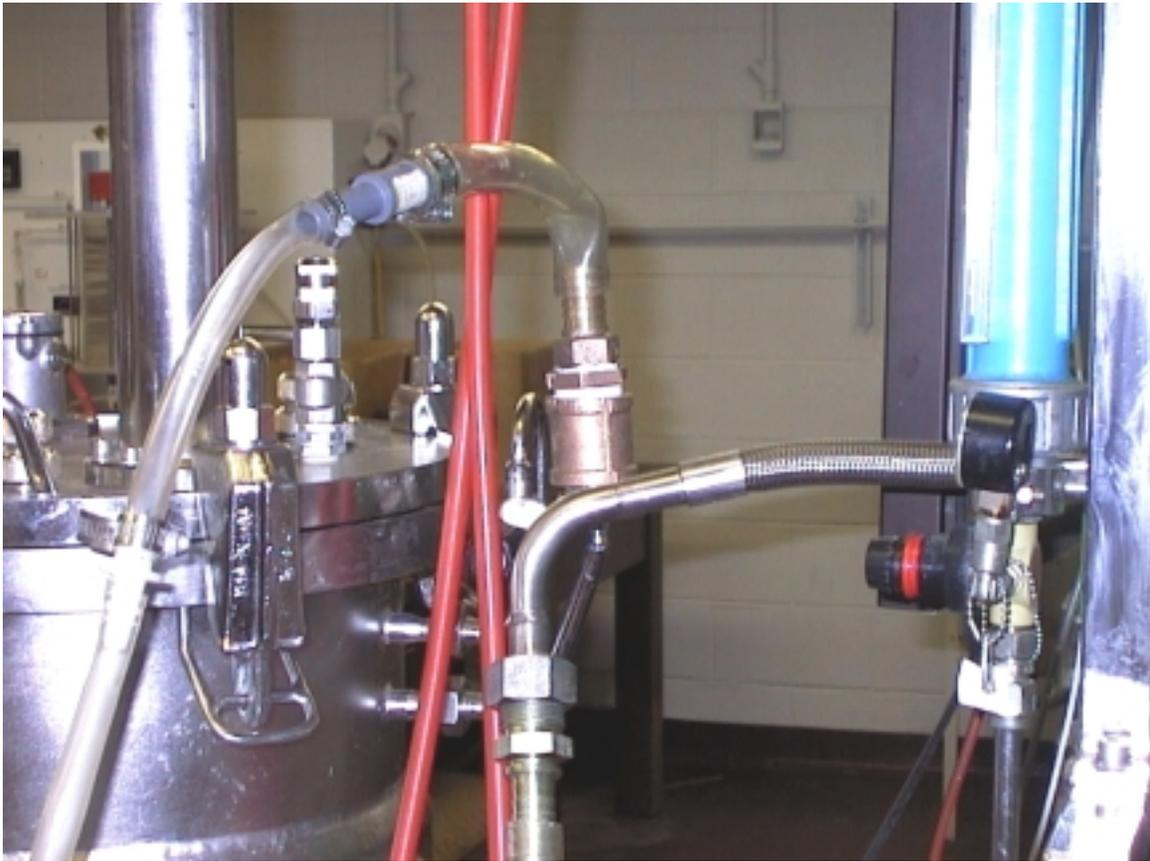
Figure 3.3 The brass hose barb connected to the air connection.
