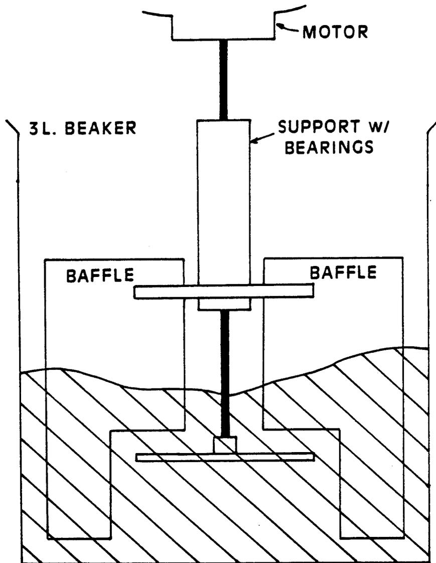
Figure 2.8 The spinning disk CGA generator (Sebba, 1985).
