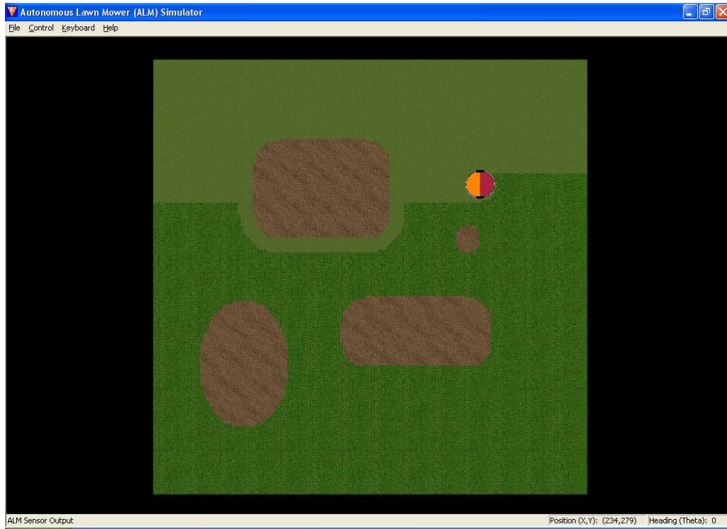
Figure 3.10: The ALM traversing its calculated optimal path
