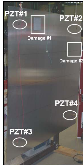
Figure 4.2.6: Ovals mark the PZT locations and squares mark the corrosion damage locations.
