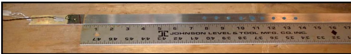
Figure 3.2.2: The aluminum beam used in the corrosion coverage test in its final damage state.
