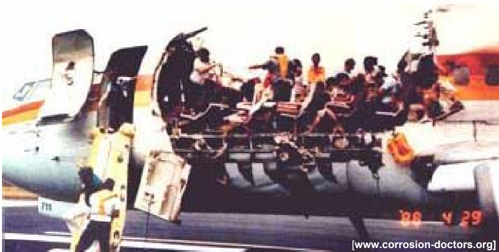
Figure 1.1.2: Corrosion induced in-flight failure in an Aloha Airlines 737 [1].
