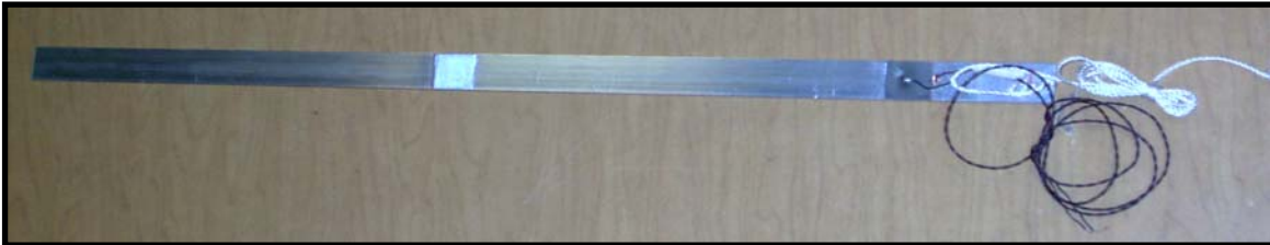
Figure 3.2.1: The beam used for pit depth detection after 5 levels of corrosion damage.
