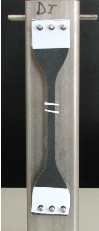
Figure 5: Custom built screening fixture used to prescribe held strain on samples
