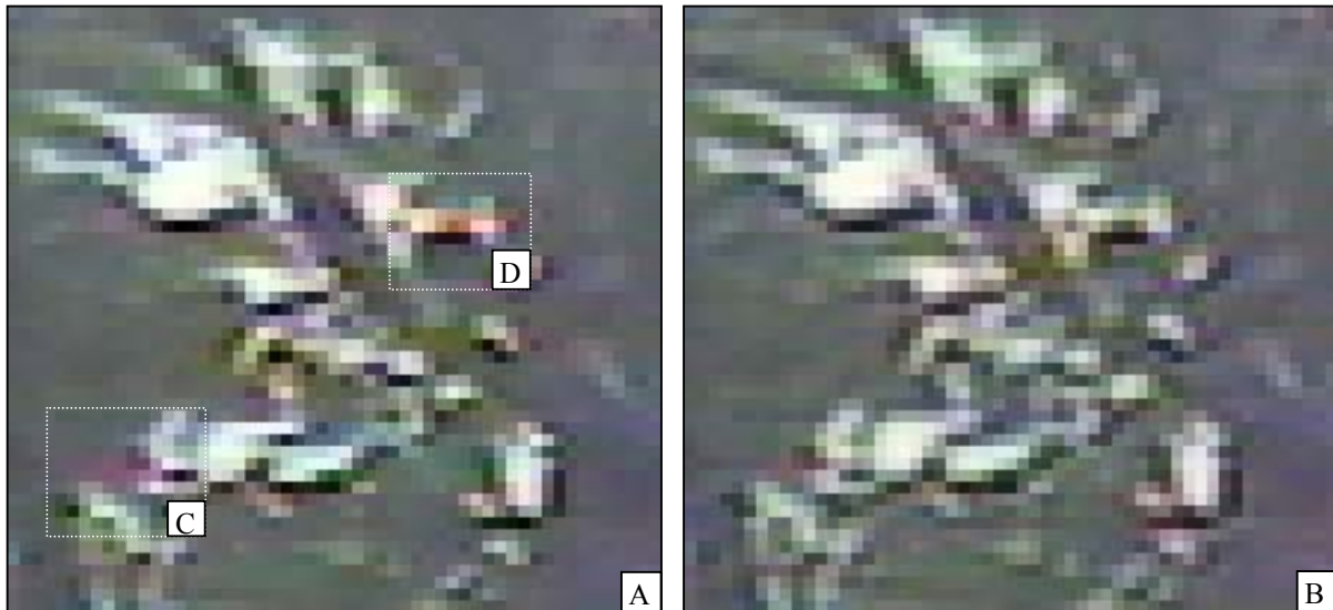
Figure 4.33: A) Mosaic 252evn contains CCD artifacts at high-contrast edges prior to Step 6. B) Mosaic 251evn after Step 6. CCD artifacts, pixel bleeding and spectral effects are reduced in image B. Pixel bleeding at C and D is reduced after Step 6.
