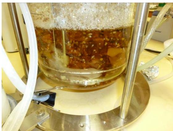
**Figure 4- 4.** Batch fermentation of *P. irregulare* with a baffle and an agitation speed of 150 rpm.
