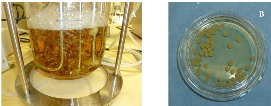
**Figure 4- 5.** Batch fermentation of *P. irregulare* without a baffle and an agitation speed of 150 rpm. (A) fermentor. (B) pellets.
