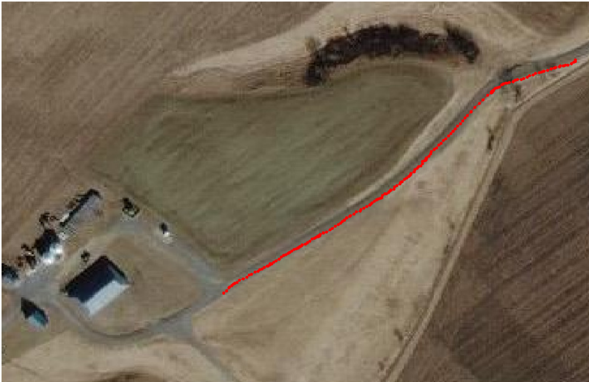
Figure 4.2: The track of the ATV during a test run as recorded with the GPS unit.
