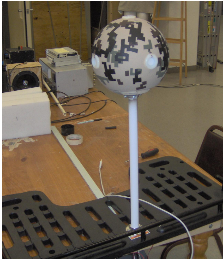
Figure 3.6: 5-microphone array shown mounted to front equipment rack.
