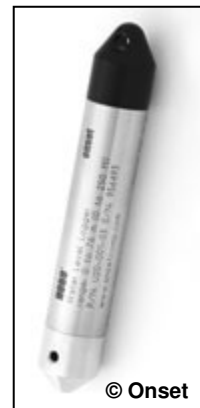
Figure 4.10. Hobo U20 pressure transducer used in the piezometers.
