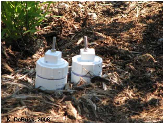
Figure 4.9. Uphill piezometer set for the structural soil infiltration trench.
