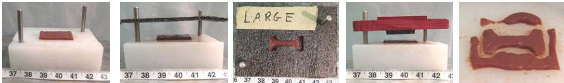
Figure 17: Specimen Stamping Methodology
