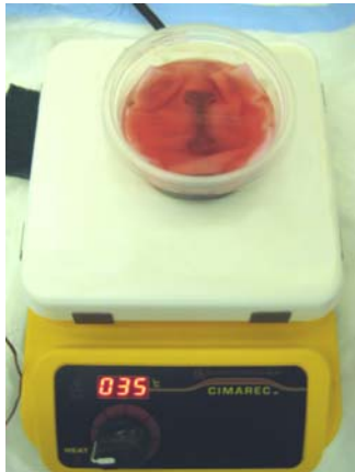
Figure 18: The hot plate warms the tissue to approximately 37°C
