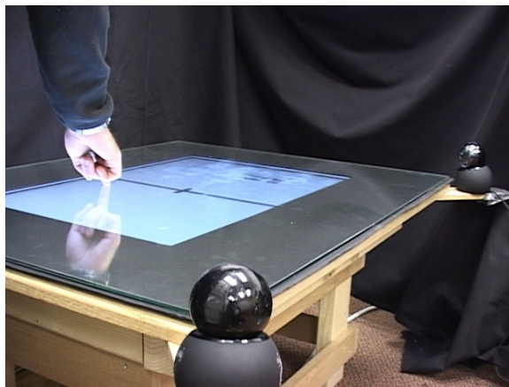
Figure 1.3: Tabletop ‘MirrorTrack’ setup, two side-mounted cameras next to the screen
