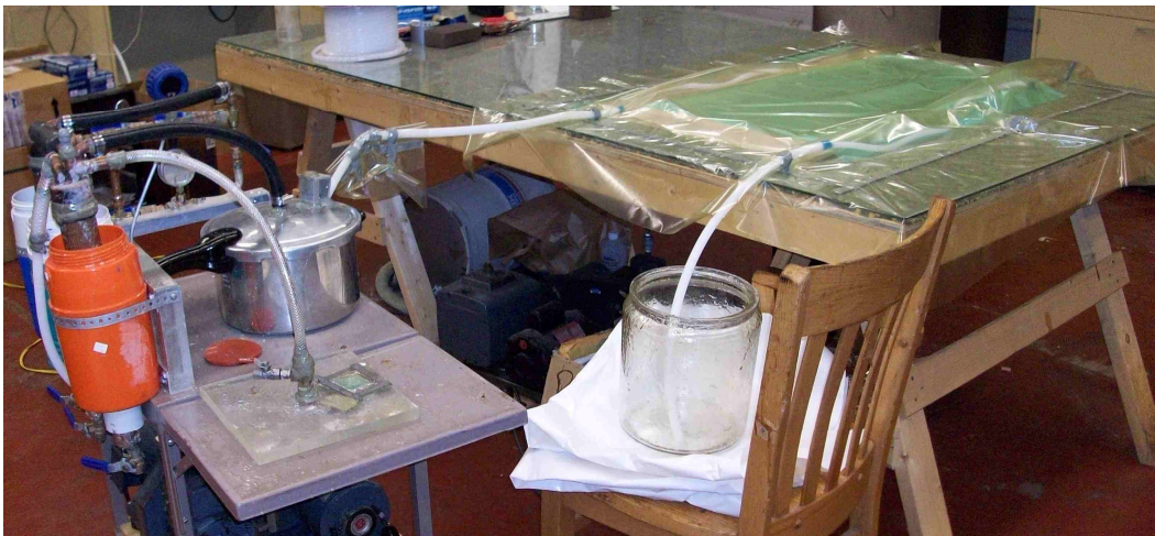
Figure 29. E-glass fabric layup in VARTM vacuum bag prior to resin infusion.
