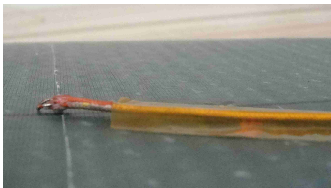
Figure 23. Thermocouple attachment at the unexposed surface showing slight arching of thermocouple wire before bead prior to insulating with silicone.
