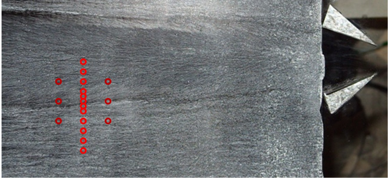
Figure 2.6.1 Flow Visualization with Approximate 10.5 cm Plane Measurement Locations
