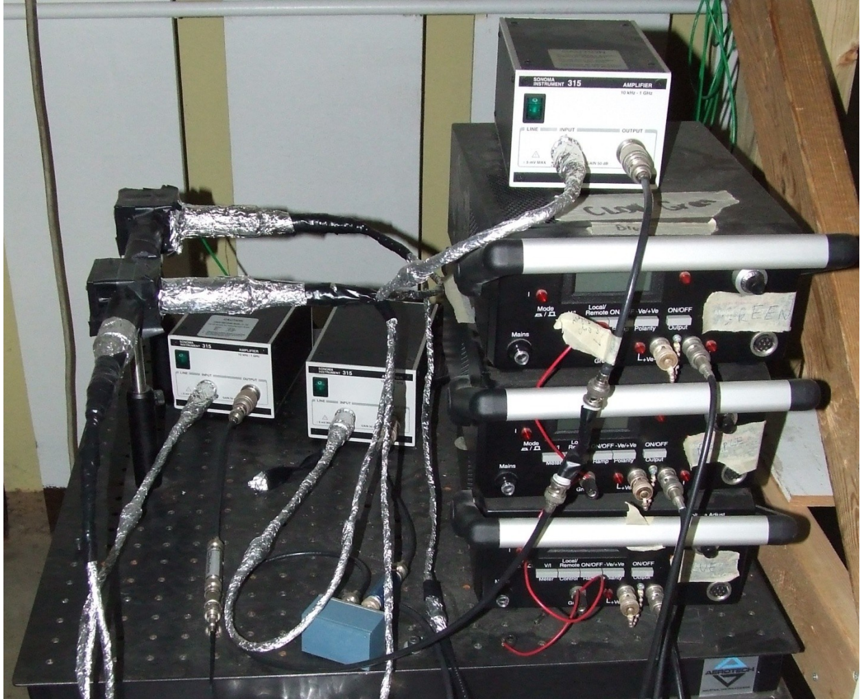
Figure 2.8.3 PMT Array, Amplifiers, and Power Supplies
