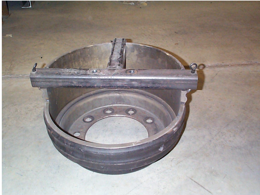
Figure 3-7 Modified Brake Drum for Kinematics Tests.
