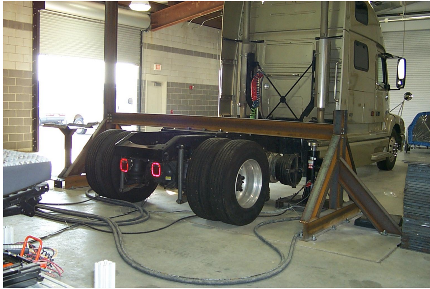
Figure 3-6 Structure for Grounding Vehicle Frame During Kinematics Tests.
