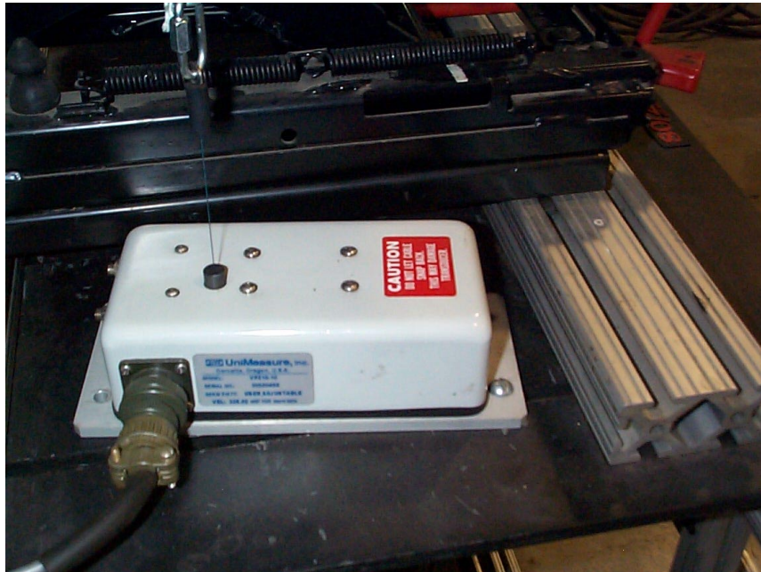
Figure 3-12 Unimeasure VP510-10-NJC LVDT.
