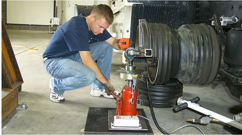
Figure 3-9 Actuation System for Kinematics Tests, Attached to Vehicle.
