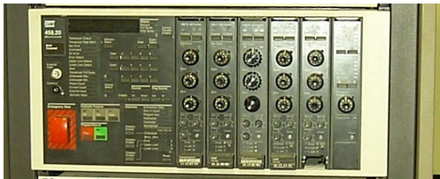
Figure 3-15 MTS 458.20 Hydraulic Controller.
