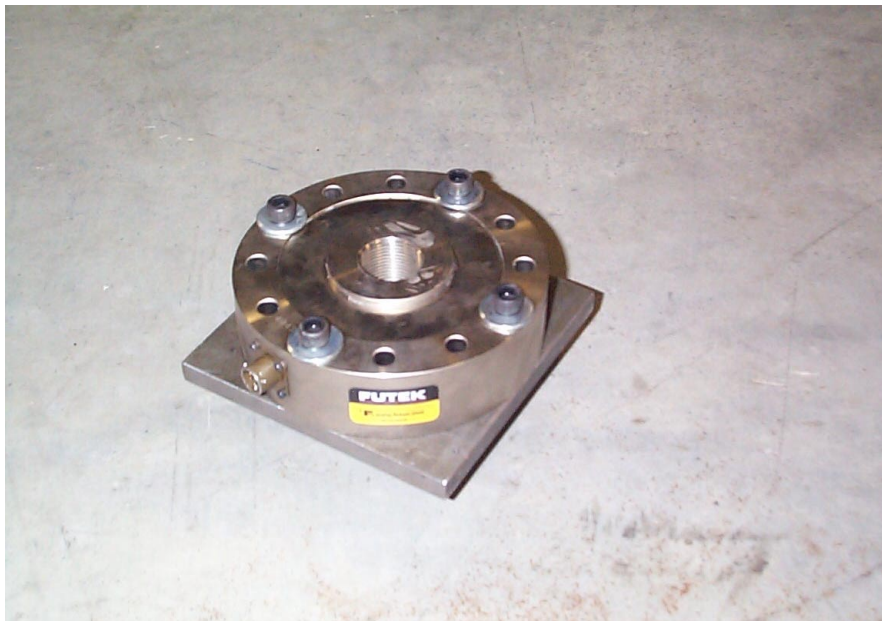
Figure 3-11 Futek Model L2900 Load Cell with Attachment.
