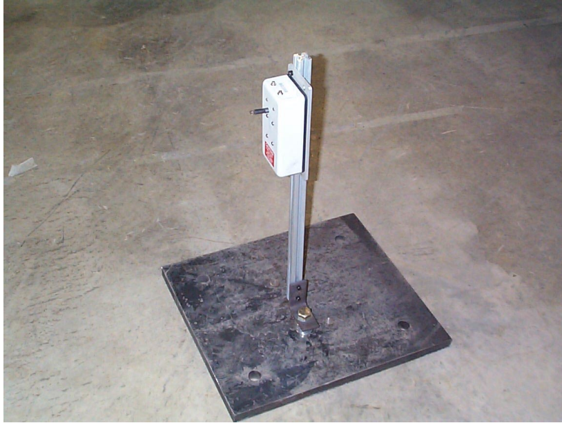
Figure 3-13 Longitudinal and Lateral Displacement LVDT Stand.
