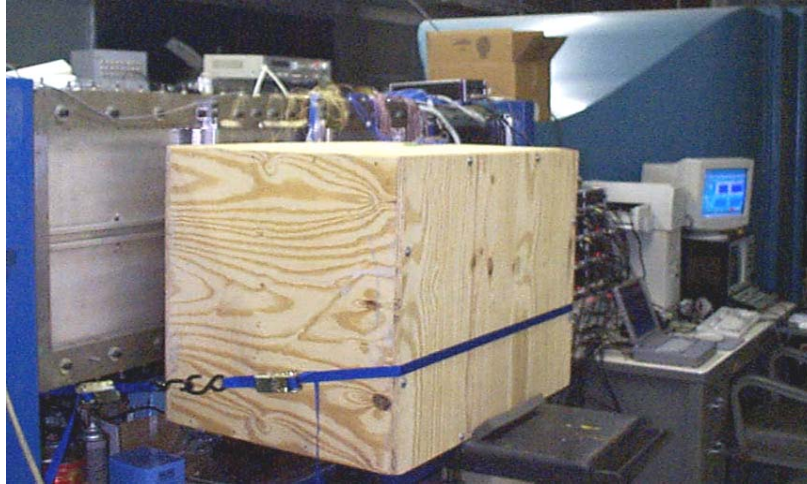
Figure 5.7 NASA LaRC panel with anechoic enclosure mounted in place.
