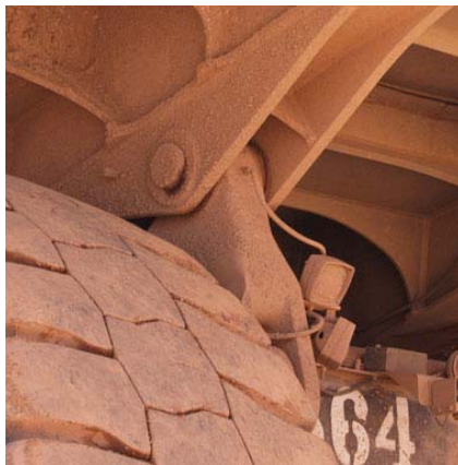
Figure 4.27 - Actual Pivot Joints
