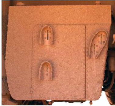
Figure 4.35 - Actual Hydraulic Tank
