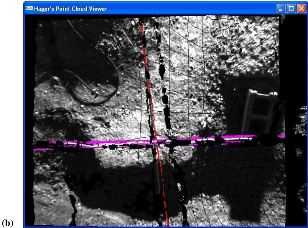
Figure B.20 Scene Cross_90_2. (a) Input range image. (b) Utility cable detection output.
