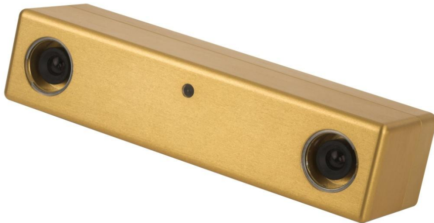
Figure 1.2 Bumblebee stereo vision camera system
