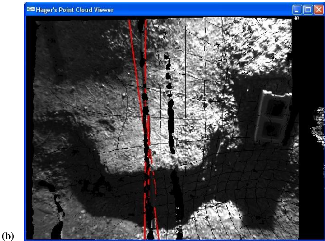
Figure B.9 Scene 90_H1. (a) Input range image. (b) Utility cable detection output.
