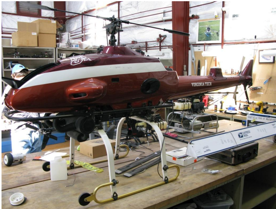
Figure 1.7 RMAX helicopter to be used on missions
