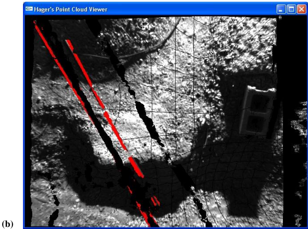
Figure B.8 Scene 60_H2. (a) Input range image. (b) Utility cable detection output.
