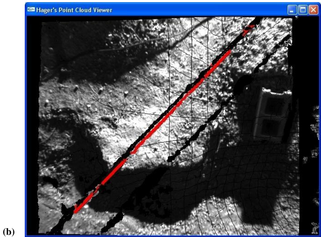
Figure B.14 Scene 135_H2. (a) Input range image. (b) Utility cable detection output.
