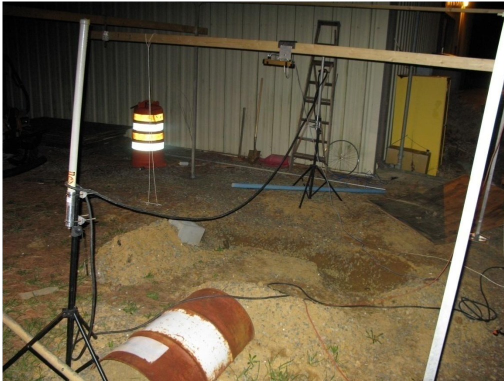
Figure 3.10 Utility cable simulation setup; camera setup can be seen near top of photo
