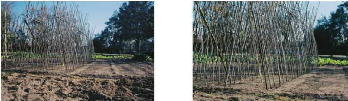
Figure 4.9 Comparison of images taken of same scene with 75^\circ (left) and 47^\circ (right) HFOV angles
