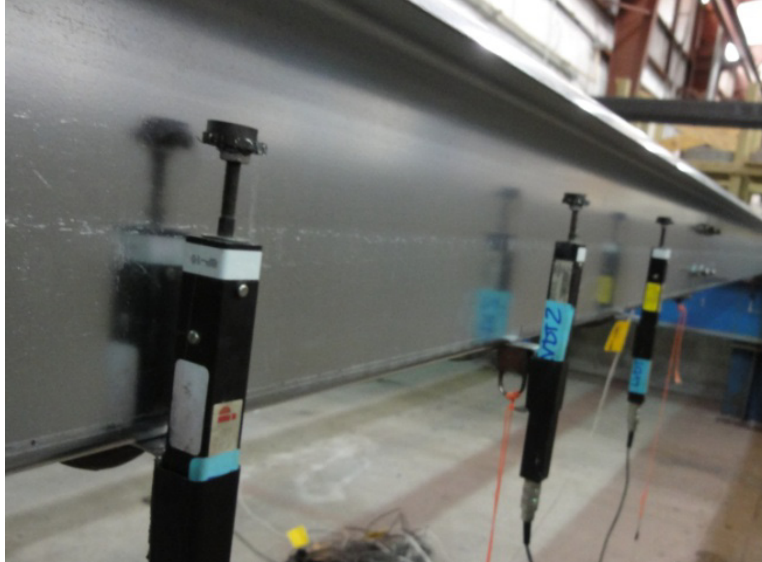
Figure 6.6 Distortional buckling LVDTs
