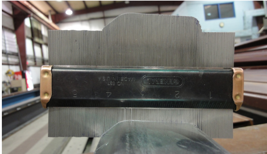
Figure 6.7 Specimen measuring - contour gauge
