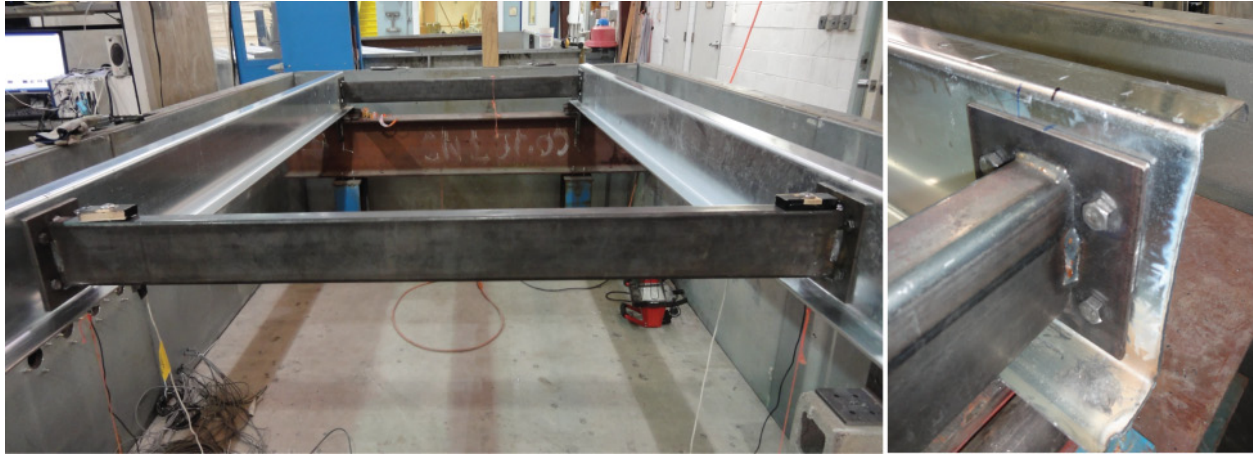
Figure 6.3 Bracing provided for lateral-torsional buckling prevention
