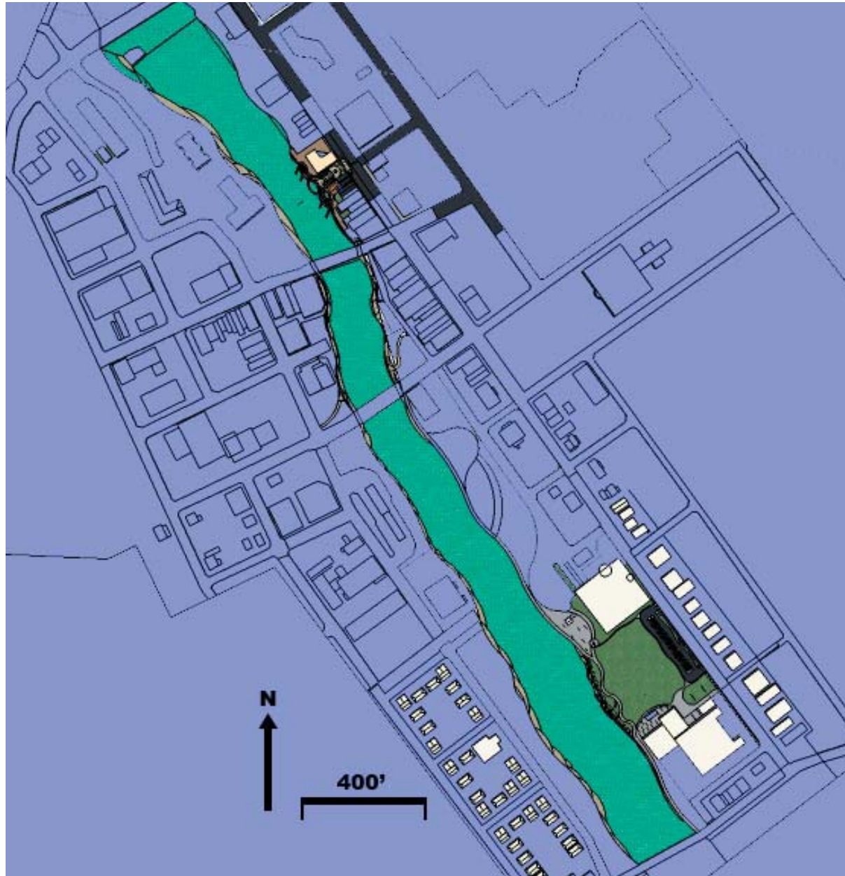
Figure 8.8. The plan view of the river shows the new curvilinear bank.
