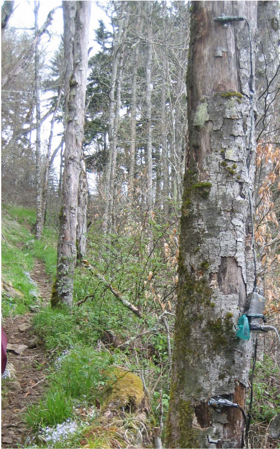
Figure 3.4. Example of TRAFx mechanical counter installation with dual sensor scopes
