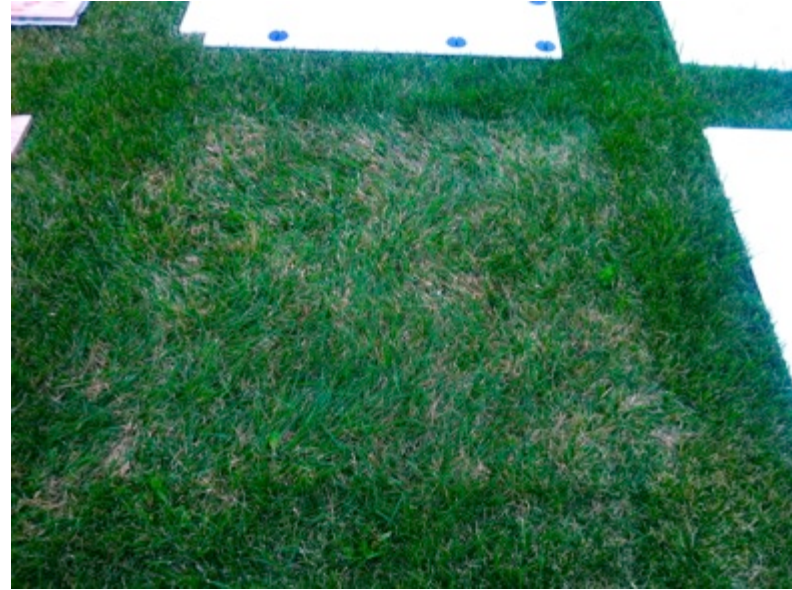
Figure 10. Symptoms of high temperature stress on tall fescue after eight days under Terratile (left) and Matrax (right) in summer 2011.
