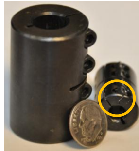
Figure 18: Rigid Coupling Replacement
